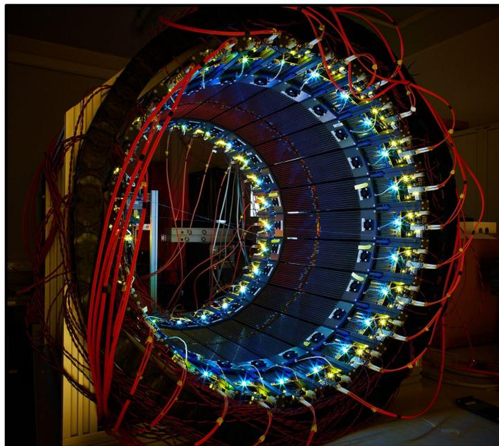
Fig. 2 The system is composed of 24 modules, each is build out of 50 cm long 13 scintillator strips, read out by a SiPM matrix.
