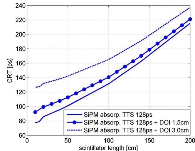
Fig. 4 CRT values as a function of the AFOV expected while using BC-408 scintillator. Values obtained for the radial thickness of 1.5 cm and 3.0 cm, in the case of unknown DOI, are indicated by a solid line with dots and a dotted line, respectively. The result for ideal case with a known DOI is shown by a solid line.
