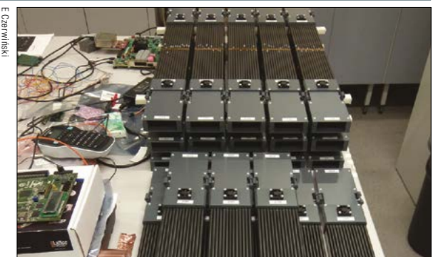
Fig. 2. Scintillator for a new J-PET layer with attached silicon photomultiplier (left), and modules consisting of 13 scintillators ready for implementation as a fourth J-PET layer (right).
