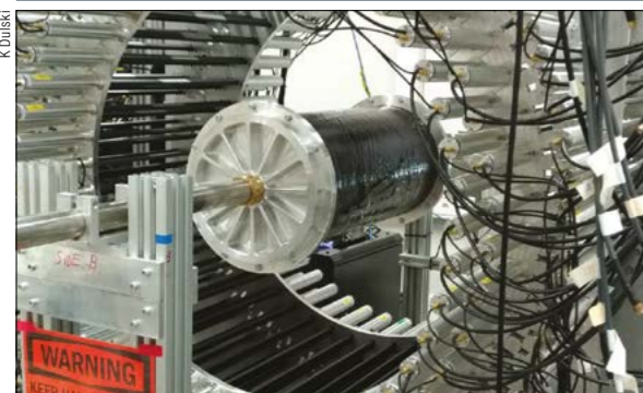
Fig. 1. (Left) The J-PET setup with a vacuum chamber installed in the centre for physics research. (Right) The position of a positronium annihilation event in the wall of a cylinder (green) can be reconstructed based on the position and time of the registered annihilation gamma quanta ( k_1, k_2, k_3 ). Since the polarisation direction of a positron emitted from a beta source is mostly preserved during positronium formation, the positronium spin direction ( S ) can also be obtained from the known positron emission point (centre) and the reconstructed e^+e^- annihilation point.
