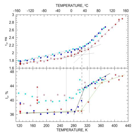
Figure 32 Temperature dependence of ortho-positronium lifetime ( $\tau_3$ ) and intensity ( $I_3$ ) in J-PET scintillator based on polyvinyltoluene (stars) and pure polyvinyltoluene (dots). Red stars refer to J-PET scintillator when heating, pink ones, when cooling. Dark blue dots refer to pure polyvinyltoluene when heating, light blue dots, when cooling down.
