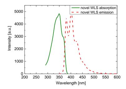
Figure 11 Absorption and emission spectra of 2-(4-styrylphenyl)benzoxazole. Absorption spectrum (solid green line) was registered with Hitachi U-2900 Spectrophotometer, and emission spectrum (red dashed line) by Hitachi Fluorescence Spectrophotometer F 7000, the plot was corrected by the detector sensitivity.
