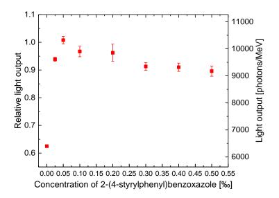
Figure 19 Relative and absolute light output of J-PET plastic scintillators. The relative light output was determined with respect to the BC-420 plastic scintillator.
