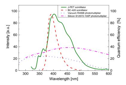
Figure 15 Emission spectra of J-PET (green solid line) and BC-420 [12] (red dashed line) scintillators superimposed on the quantum efficiency dependence on photons wavelength for typical vacuum tube photomultiplier with bialcali window (blue dotted line) [21] and silicon photomultipliers (pink dashed-dotted line) [21]. Maximum of emission for BC-420 scintillator is placed at wavelength of 393 nm, while the maximum of J-PET scintillator at 403 nm. The emission spectra are normalized in amplitude.
