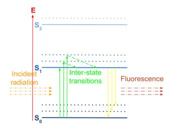
Figure 4 Scheme of the singlet energy level diagram of organic scintillators [33].
