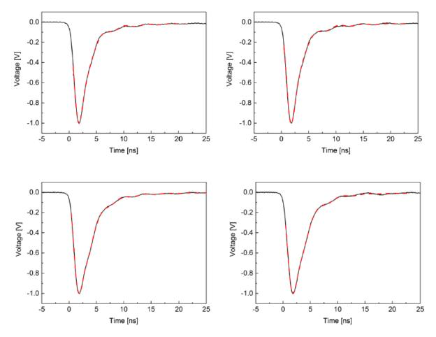
Figure 21 Averaged signals from photomultiplier connected to BC-420 (top panel) and J-PET scintillator (bottom panel). Superimposed dashed-red lines indicate result of the fitting of sum of functions given by formulas 4 and 5. Signals were normalized to 1 V.
