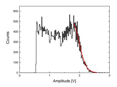
Figure 7 Amplitude spectra of stilbene with Fermi function fitted (red).
