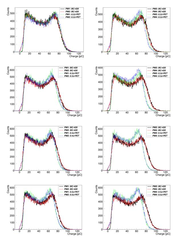
Figure 18 Charge spectra registered for BC-420 and J-PET scintillators. PM1, PM2, PM3 and PM4 denote particular photomultipliers, according to Fig. 17. Spectra are registered for J-PET scintillators containing different amounts of novel wavelength shifter, from 0 to 0.5 ‰. Names of scintillators refer to the amount of wavelength shifter. In the left panel spectra registered by PM1 and PM2 for BC-420 and J-PET are presented, while in the right panel spectra registered by PM3 and PM4 are given.
