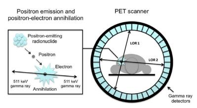
Figure 1 The scheme of positron - electron annihilation (left) and PET scanner (right). Figure is adapted from [3].
