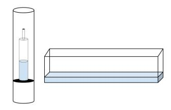
Figure 35 Left panel: the scheme of arrangement of glass ampoule in pipe furnace. Right panel: the scheme of arrangement of the form in DCF420/spec furnace. Figure is not to scale, the volume of scintillator is marked in blue.
