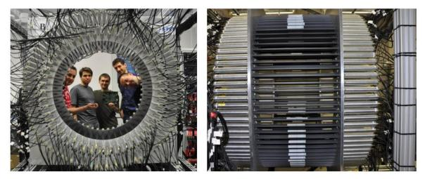
Figure 3 A front (left) and side (right) view of J-PET scanner prototype [23]. Scintillators wrapped in the black foil are placed in the middle. At their both ends vacuum photomultipliers are connected. Photomultipliers are placed inside lightproof aluminum housings.
