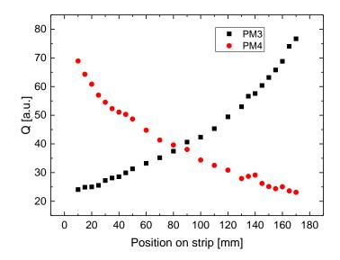
Figure 38 Charge (Q) of signals at Compton edge for irradiation positions along the J-PET scintillator strip. Charge was calculated for signals registered by photomultipliers at both ends of scintillator (PM3 and PM4).
