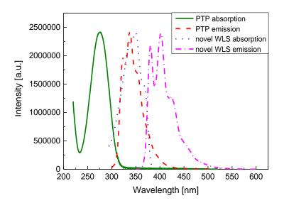
Figure 14 Absorption and emission spectra of p-terphenyl (PTP) are marked with green solid line and red dashed line, respectively. Spectra are taken from [69]. Absorption and emission spectra of 2-(4-styrylphenyl)benzoxazole (novel WLS) are marked with blue dotted line and pink dashed-dotted line, respectively.
