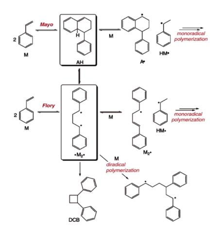
Figure 8 Mayo's and Flory's mechanisms of free radical generation in styrene polymerization. The scheme is taken from the article [61].
