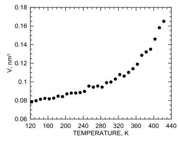
Figure 31 The size of spherical free volume as a function of temperature in scintillator based on polystyrene, containing 2 % of PPO and 0.03 % of 2-(4-styrylphenyl)benzoxazole.
