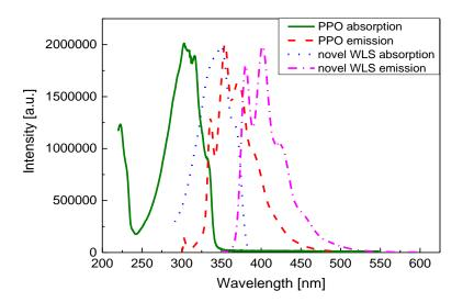
Figure 13 Absorption and emission spectra of 2,5-diphenyloxazole (PPO) are marked with green solid line and green dashed line. Spectra are taken from [69]. Absorption and emission spectra of 2-(4-styrylphenyl)benzoxazole (novel WLS) are marked with blue dotted line and pink dashed-dotted line, respectively.
