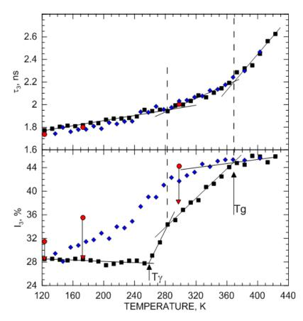
Figure 29 Temperature dependence of  $I_3$  in J-PET plastic scintillator. Points denote: squares - increasing temperature; diamonds - decreasing temperature; dots and triangles - first and last points in the measurements of irradiation effect; dashed lines and arrows denote the transition temperatures; red dots with arrows denote sections of time relaxation.
