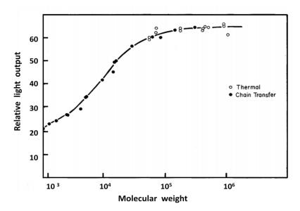
Figure 22 The influence of molecular weight on the relative light output of plastic scintillators. Filled dots refer to samples in which molecular weight were changed by chain transfer agents, while empty dots refer to samples in which molecular weight was changed by polymerization temperature. The figure is adapted from [84].
