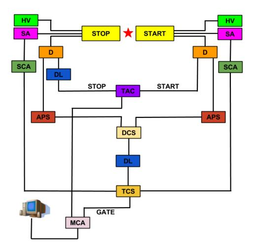
START - detector registering gamma quanta with energy of 1274 keV
