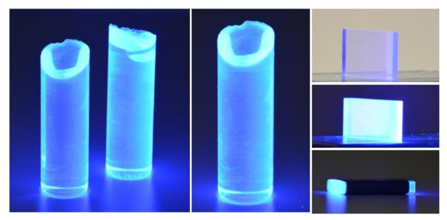
Figure 10 J-PET plastic scintillators in UV light. Left and centre: scintillators removed from the glass ampoule. Right from the top: scintillator cut and polished, exposed to UV in daylight, in the dark and scintillator wrapped in light tight foil in the dark.
