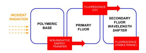
Figure 5 Block scheme of energy transfer in plastic scintillator.
