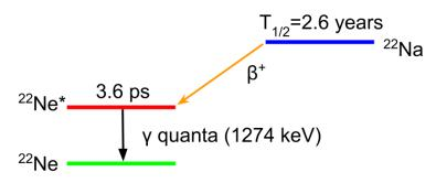
Figure 27 The scheme of <sup>22</sup>Na source decay in which gamma quanta of energy 1274 keV are produced just after emission of positron. Gamma quanta production is preceded by creation of non stable excited state of <sup>22</sup>Ne.
