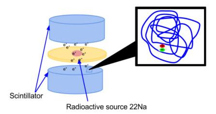
Figure 25 The scheme of plastic scintillators samples arrangements in the experimental setup. Positrons emitted from sodium source interact with scintillating material forming positronium atom in empty voids between and around polymeric chains.
