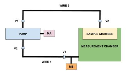
Figure 26 Block scheme of the vacuum part of the experimental setup for positronium lifetime measurements. V1 and V2 denote valves, MA and MB denote measurers of vacuum.
