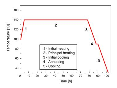
Figure 9 Temperature schedule of the plastic scintillators polymerization [68].
