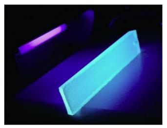
Figure 37 J-PET scintillator strip exposed to UV light.
