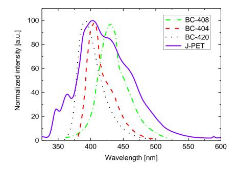
Figure 40 Emission spectra of BC-408 (green dashed - dot line), BC-404 (red dashed line), BC-420 (black dotted line) and J-PET scintillator (violet solid line).
