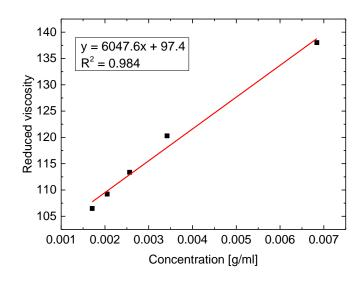
Figure 24 Determination of intrinsic viscosity for a polystyrene solution in toluene.
