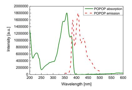
Figure 12 Absorption (green solid line) and emission (red dashed line) spectra of POPOP in cyclohexane [69].
