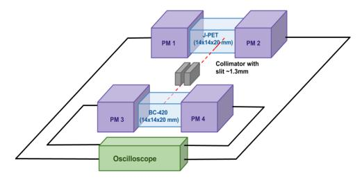
Figure 17 A scheme of experimental setup used to determine J-PET scintillators light output. Performance of J-PET scintillator was compared to BC-420 scintillator. Detailed description of the setup and experimental procedure is given in the text.
