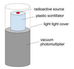
Figure 6 Experimental setup for the estimation of plastic scintillators light output.
