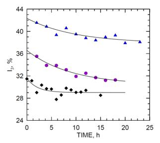
Figure 30 The ortho-positronium intensity ( $I_3$ ) dependence on time in temperatures: 123 K (black diamonds), 173 K (violet dots) and 298 K (blue triangles) in scintillator based on polystyrene, containing 2 % of PPO and 0.03 % of 2-(4-styrylphenyl)benzoxazole.
