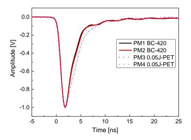
Figure 20 Average signals appearing in 0.05J-PET and BC-420 scintillator, normalized to the amplitude of 1 V. PM denotes particular photomultiplier.
