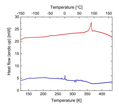
Figure 34 Thermogram of pure polyvinyltoluene. Red line denotes heating, blue one cooling of the sample.
