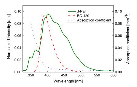
Figure 16 Emission spectra of J-PET (green solid line), BC-420 scintillator (red dashed line) and absorption coefficient  $\mu_{eff}$  (blue dotted line) [70] [71]. The emission spectra are normalized in amplitude.
