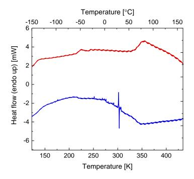
Figure 33 Thermogram of J-PET scintillator containing 0.05 ‰ of novel WLS. Red line denotes heating, blue one cooling of the sample.
