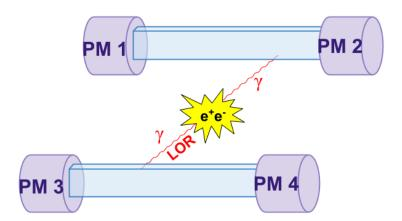
Figure 2 Scheme of the simplest unit of J-PET scanner. PM denotes photomultiplier.
