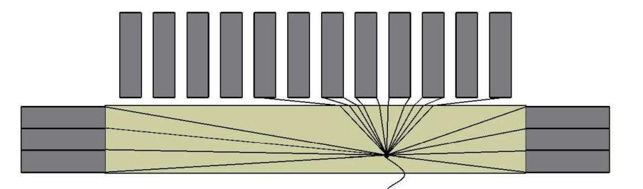
Even though the single detection block will be large, the proposed concept of Matrix-PET detector will allow to determine the depth of interaction. Depth at which gamma quantum has been absorbed will be determined based on amplitudes distribution of signals from left-right and front-rear photomultipliers. Section of scintillator plate with photomultipliers is shown above.
