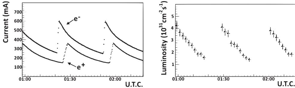
Fig. 3. – Left: beam currents measured by the SIDDHARTA-2 luminometer during the first collision tests. Right: instant luminosity with time intervals of 120 s [10].
