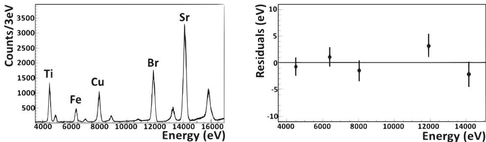
Fig. 2. – Left: example of an SDD calibrated spectrum collected with an X-ray tube, during the DAΦNE beam commissioning phase. Energy resolution at 170 K for the Fe  $K_{\alpha}$  line is  $166 \pm 4$  eV. Right: the linear response of SDDs system is  $\Delta E/E < 10^{-3}$  in the range of 4000–14000 eV.
