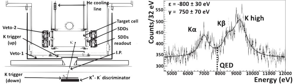
Fig. 1. – Left: cross section layout of SIDDHARTA-2 setup. Right: Monte Carlo simulation of K<sup>-</sup>d corresponding to an integrated luminosity of  $800 \text{ pb}^{-1}$  (with input  $\epsilon_{1s} = -800$  eV,  $\Gamma_{1s} = 750$  eV and yield = 0.1%). Dot line at 7834 eV refers to the pure QED  $K_{\alpha}$  value.
