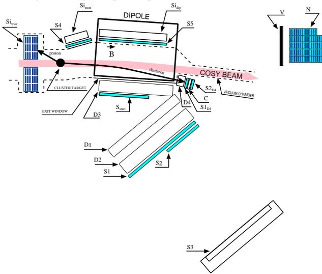
Fig. 1: Schematic view of COSY-11 detection setup. D1, D2, D3 and D4 denote the drift chambers; S1, S2, S3, S4, S5,  $S_{start}$ ,  $S1_{D4}$ ,  $S2_{D4}$  and V the scintillation detectors; C Cerenkov counter; N the neutron detector and  $Si_{mon}$ ,  $Si_{spec}$  and  $Si_{dip}$  silicon strip detectors to detect elastically scattered, spectator protons and negatively charged particles, respectively.
