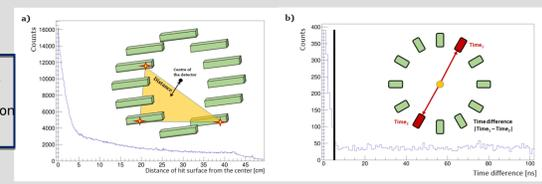
Fig. 6. (a) Next criteria is checking coplanarity of annihilation hits. Because source with material was in the center of the detector the distance of decay plane from the center should be close to zero. (b) Next condition selecting true annihilations is checking the time difference between annihilation hits, knowing that the annihilation should take place in the center.
