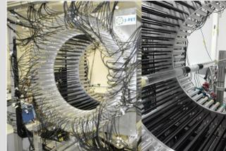
Fig. 3. Photo of J-PET scanner front view (right), sample with  $^{22}\text{Na}$  source sealed in Kapton foil inside the scanner (left).
