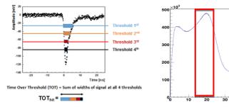
Fig. 4. (left) The Time-Over-Threshold (TOT) values are calculated and used as a measure of Energy. (right) Applied cut on TOT: Annihilation 14-24 ns, deexcitation 35-55 ns.
