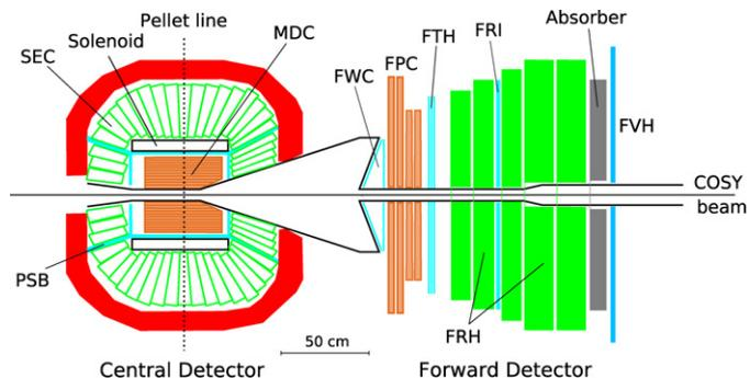
Fig. 2. Schematic side view of the WASA detector setup at COSY.
