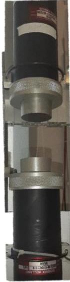
Fig.17. PALS setup consisting of two BaF2 detectors aligned in a collinear manner
