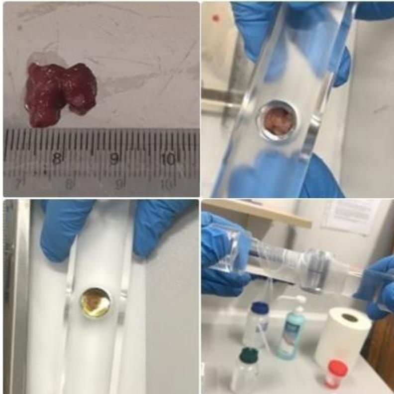
Fig.20. Photographs illustrating sample preparation and mounting in chamber with radioactive source. Firstly the sample is cutted, then placed in holder with the source and at the end siled with paralim [45].
