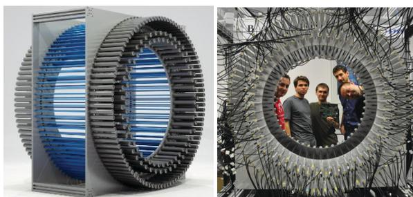
**Figure 2.** (Left) Visualization of the J-PET detector prototype. One can see three layers of scintillator strips connected with photomultipliers and arranged in a barrel. (Right) Photograph of the first prototype of the J-PET detector together with few members of the collaboration.
