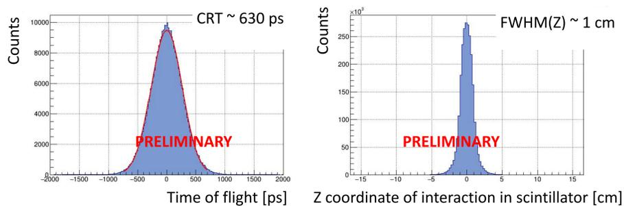
Fig 2. (left) Time of flight spectrum after first two iterative walk corrections. (right) Distribution of Z coordinates of interaction position inside scintillator.
