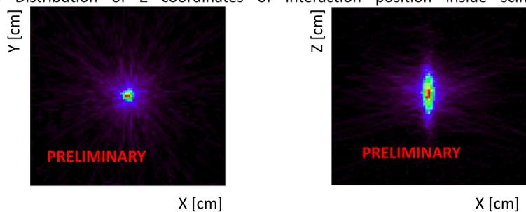
Fig 3. Point-like source image reconstructed with CASTOR software on (left) from the front view (XY plane) and (right) from the top (ZX plane).
