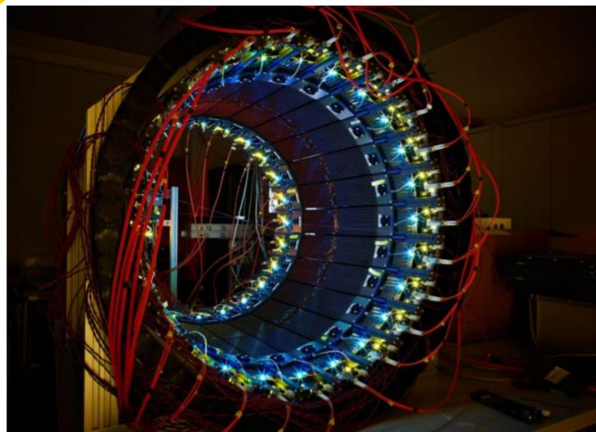
Fig 1. Mobile, modular J-PET prototype, built out of 24 modules. Each module is composed of 13 scintillator strips, read out by a SiPM array from both sides.
