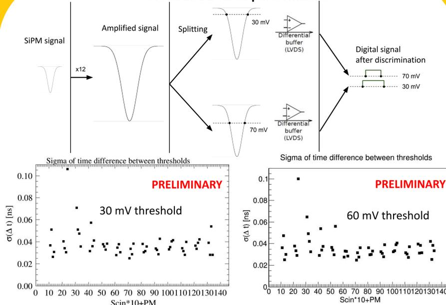
Fig 4. (top) Signal processing scheme. Each SiPM signal is amplified, then split into two and then converted with TDC unit on FPGA chip. (bottom) Time difference between two thresholds set on the same value for each SiPM.
