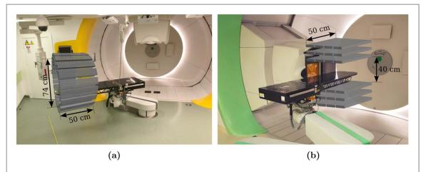
$\label{permutation} \textbf{Figure 1.} \ The proposed J-PET geometries: (a) \ the \ double-layer, full-ring \ J-PET geometry for the in-room protocol; (b) \ the \ triple-layer, dual-head \ J-PET geometry for the in-beam protocol.$
