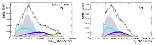
**Figure 1.** The simultaneous fit to the  $\Sigma^0 p$  invariant mass (left) and proton momentum distributions (right) performed for kaons stopped in DC wall. The colors represent the following fit contributions:  $\pi^0$  background (grey), 4NA with uncorrelated production of the  $\Sigma^0 p$  final state (cyan), 3NA (blue), 2NA-FSI (magenta) and 2NA-QF (red). The black line shows the overall fit. Figure is adopted from [24].
