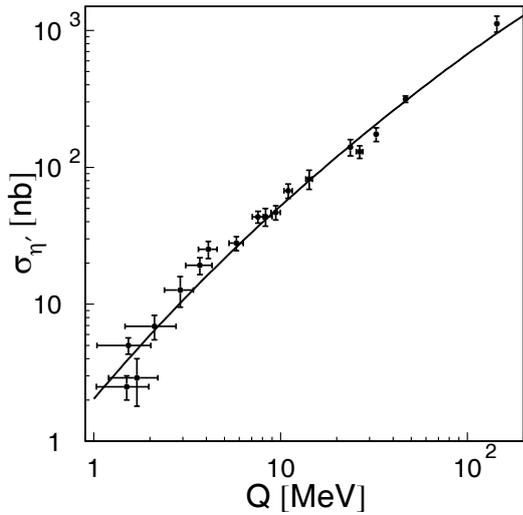
**Fig. 1.** Compilation of the data for the  $pp \rightarrow pp\eta'$  reaction cross-section from COSY-11, DISTO and SPESIII measurements [22–24,26,27]. The solid line is parameterization of the data using formula (2).
