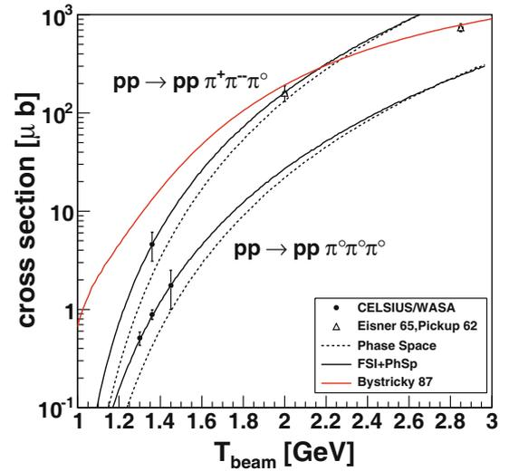
**Fig. 2.** Total cross-section for three-pion production: data and parameterizations. The data are from [43–46,32]. The parameterizations are from Bystricky *et al.* [47] and Fäldt and Wilkin [28,29]. The kinetic beam energy at thresholds for the  $\eta$  and  $\eta'$  production is equal to 1.255 GeV and 2.404 GeV, respectively.
