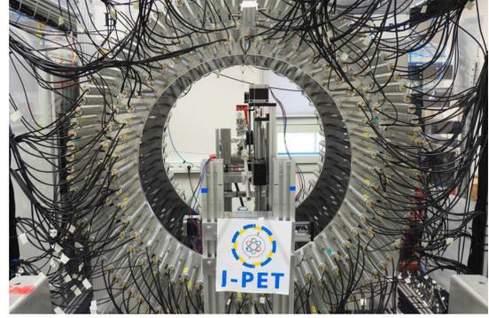
Fig. 4. The 3-layer prototype of the J-PET detector currently operating in laboratory.
