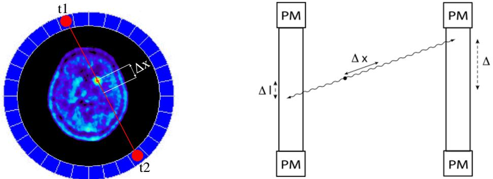
Figure 3. (Left) Illustration of the idea of PET-TOF;  $\Delta x = (t_2 - t_1) c/2$ , (Right) Schematic few of the new PET concept referred to as strip-PET. The hit position versus the center of the scintillator ( $\Delta l$ ) is determined based on time difference measured on both sides of the scintillator strip, and the position ( $\Delta x$ ) along the LOR is determined from time difference measured between two modules. PM denotes the photomultipliers.
