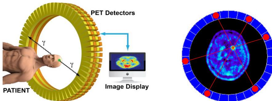
Fig. 2 (Left) Schematic view of the PET diagnostic system. (Right) Illustration of the idea of the image reconstruction. Three lines of response are indicated in red.
