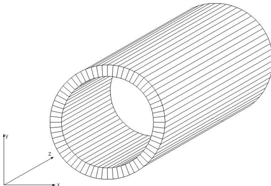
Fig. 4. Example of diagnostic chamber of the strip-PET. The chamber is formed from strips of organic scintillator.
