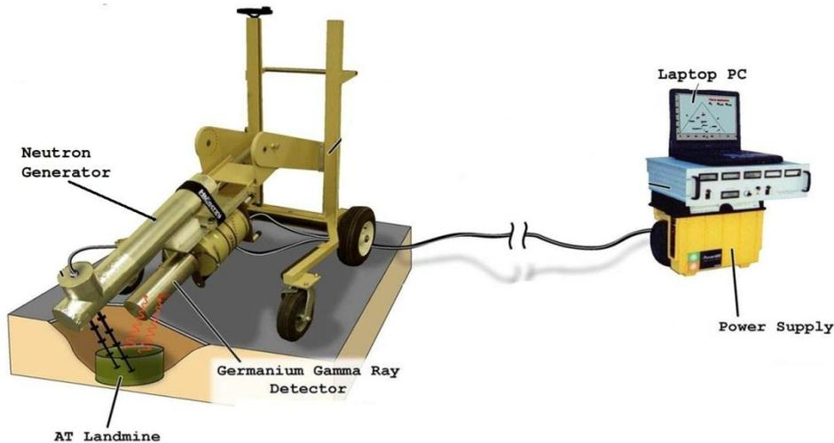
Fig. 5. Illustration of the system for explosive detection build out of a neutron generator and detector for gamma rays. In the figure only neutrons flying towards the landmine and gamma quanta towards detector are shown. In reality they are emitted isotropically in the full solid angle. The figure is adapted from [12].
