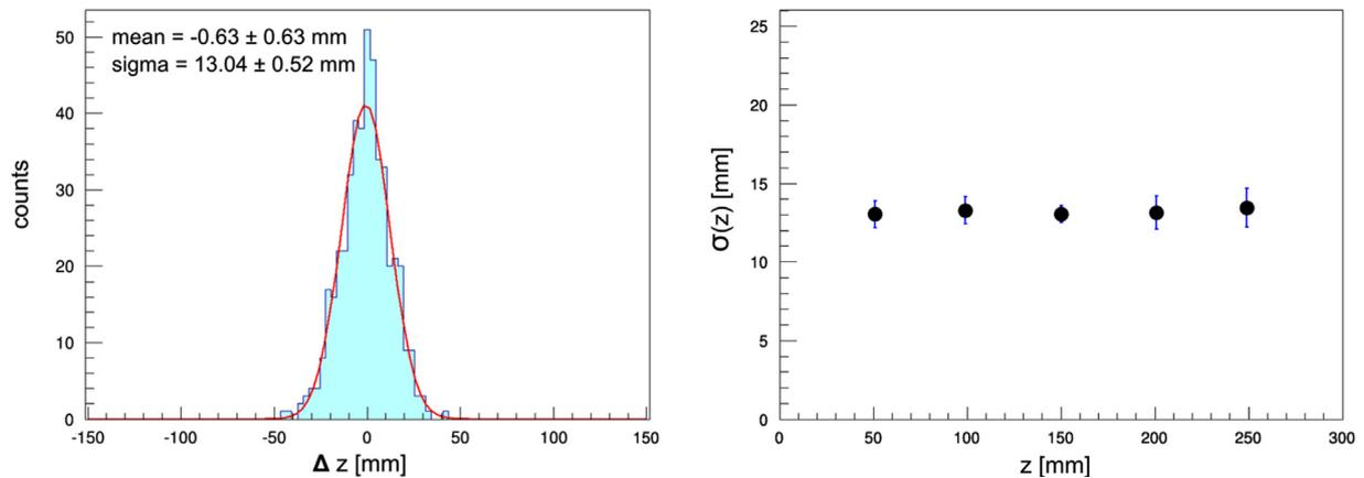
**Fig. 9.** (Left) Distribution of differences between the true and reconstructed position for signals measured at  $z=150$  mm. (Right) Position resolution as a function of the place of gamma quantum interaction.
