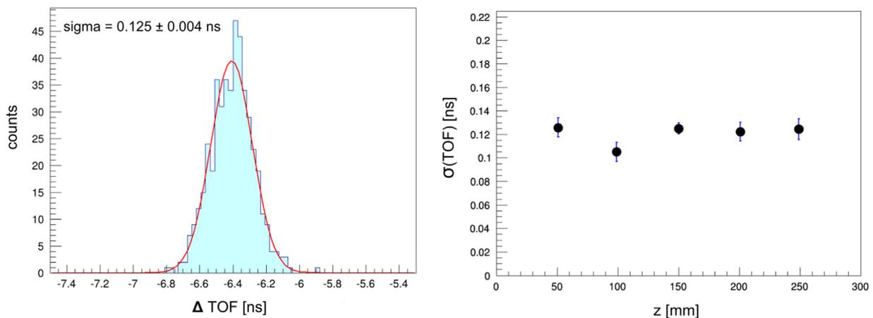
**Fig. 10.** (Left) Distribution of differences between the true and reconstructed TOF for signals measured at  $z=150$  mm. The non-zero value of the mean is mainly due to the difference in the cable lengths and it is matter of calibration. (Right) TOF resolution as a function of the place of gamma quantum interaction.
