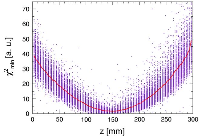
**Fig. 8.**  $\chi^2_{min}$  as a function of position assigned to the model signals. Superimposed solid line indicates average value of  $\chi^2_{min}$  determined for each position separately.
