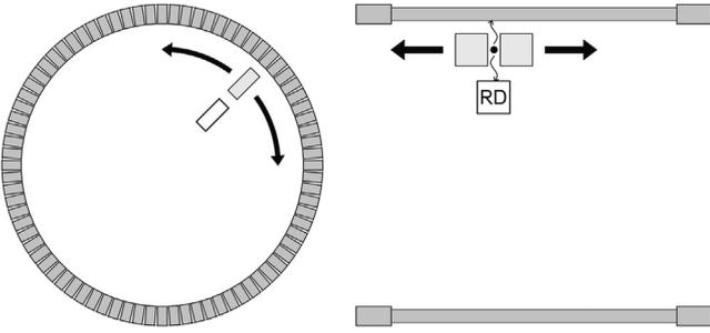
**Fig. 3.** Schematic cross-sections of the J-PET detector with a collimated beam of annihilation quanta rotating around the axis and moving along the detector, as indicated by the arrows. RD denotes a reference detector permitting to select signals corresponding to the annihilation quanta and improving the collimation.
