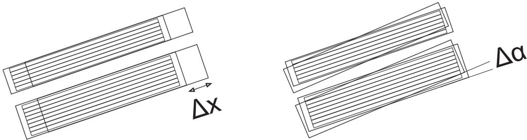
**Figure 8.1:** Schematic view (from top) with the pictorial definitions of the horizontal shift of the chambers  $\Delta x$  and their inclination  $\Delta\alpha$ . These parameters were used in the analysis to determine the proper arrangement of the D1 and D2 drift chambers relative to the COSY-11 dipole.
