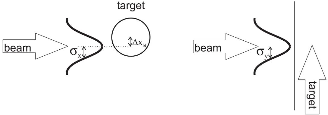
**Figure 4.5:** Schematic view of the relative target and beam settings. Left panel depicts the view from above, right presents a side view.  $\sigma_X$  and  $\sigma_Y$  denote the horizontal and vertical standard deviations of the assumed Gaussian distributions of the proton beam density, respectively.  $\Delta_{X_{bt}}$  denotes the distance between the centers of the proton target and beam. The figure is adapted from [70].
