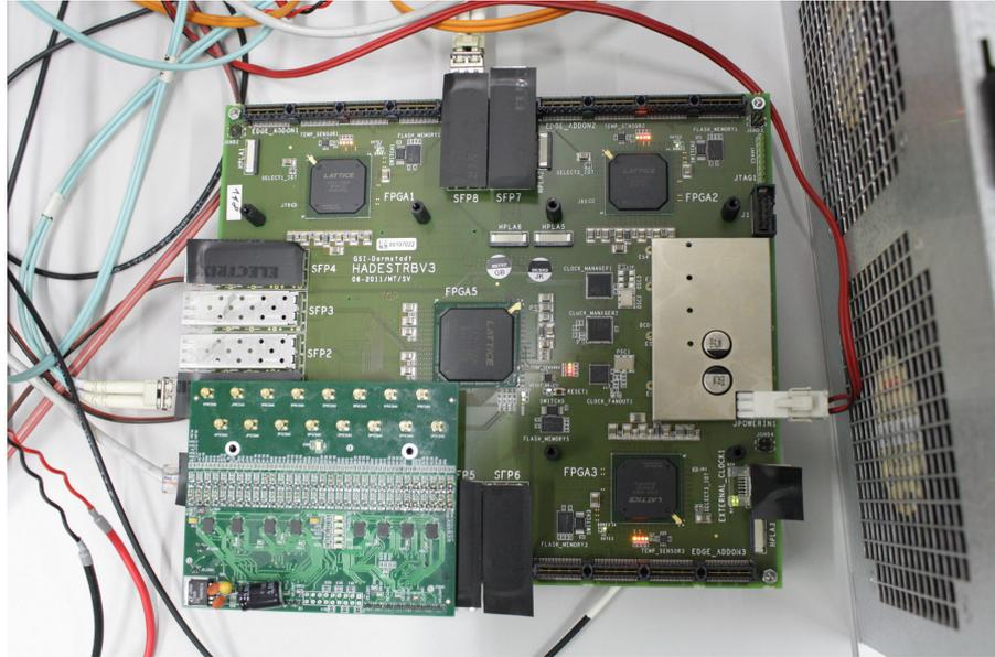
Figure 50: Next generation of multi-level constant threshold board placed on the TRB. Four of such boards could be connected to one mother board, design by M. Pałka. A single board has dimensions of  $105 \times 90 \text{ mm}^2$  and has 16 channels. Four of such boards can be connected to one TRB.
