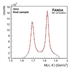
**Fig. 12** Mass distribution (black histogram) of the final reconstructed  $\Lambda$  K<sup>-</sup> from  $\bar{p}p \to \overline{\mathcal{Z}}^+ \Lambda$ K<sup>-</sup> with fit function (red dashed curve) containing two Voigt functions and a polynomial
