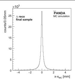
Fig. 8 Deviation of the reconstructed from the generated x coordinate of the  $\Lambda$  decay vertex in the process  $\bar{p}p \to \overline{\mathcal{Z}}^+ \Lambda K^-$  after the final selection
