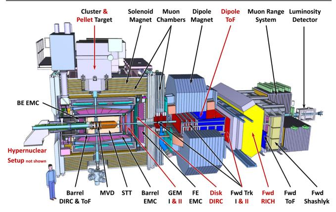
Fig. 1 Schematic overview of the  $\overline{P}$ ANDA detector setup. The components with black labels will be available for the initial configuration of  $\overline{P}$ ANDA and the components with red labels will be added later. Figure taken from [28]
