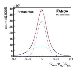
**Fig. 4** Relative momentum resolution of the reconstructed protons (black histogram). The distribution is fitted with a double Gauss fit (red dashed line). The width of the inner Gauss function (blue dashed line) is used as momentum resolution. The cyan dashed line indicates the second Gaus function
