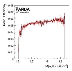
Fig. 11 Reconstruction efficiency (black histogram) as function of the invariant  $\Lambda$  K<sup>-</sup> mass in the process  $\bar{p}p \to \overline{\mathcal{Z}}^+ \Lambda$ K<sup>-</sup>. The statistical error is shown in red
