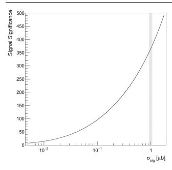
Fig. 7 Signal significance as function of the signal cross section. The gray band indicates the region the signal is assumed
