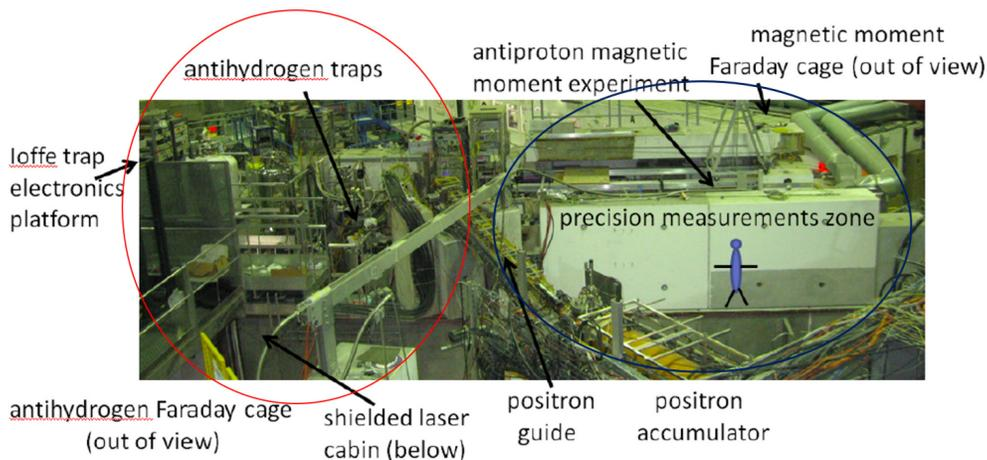
Figure 7: Photograph of the ATRAP beamline with two antiproton ports – one for antihydrogen experiments and the second for antiproton experiments.
