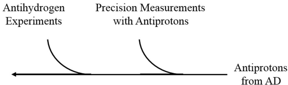
Figure 6: The ATRAP beamline has two antiproton ports – one for antihydrogen experiments and the second for antiproton experiments.
