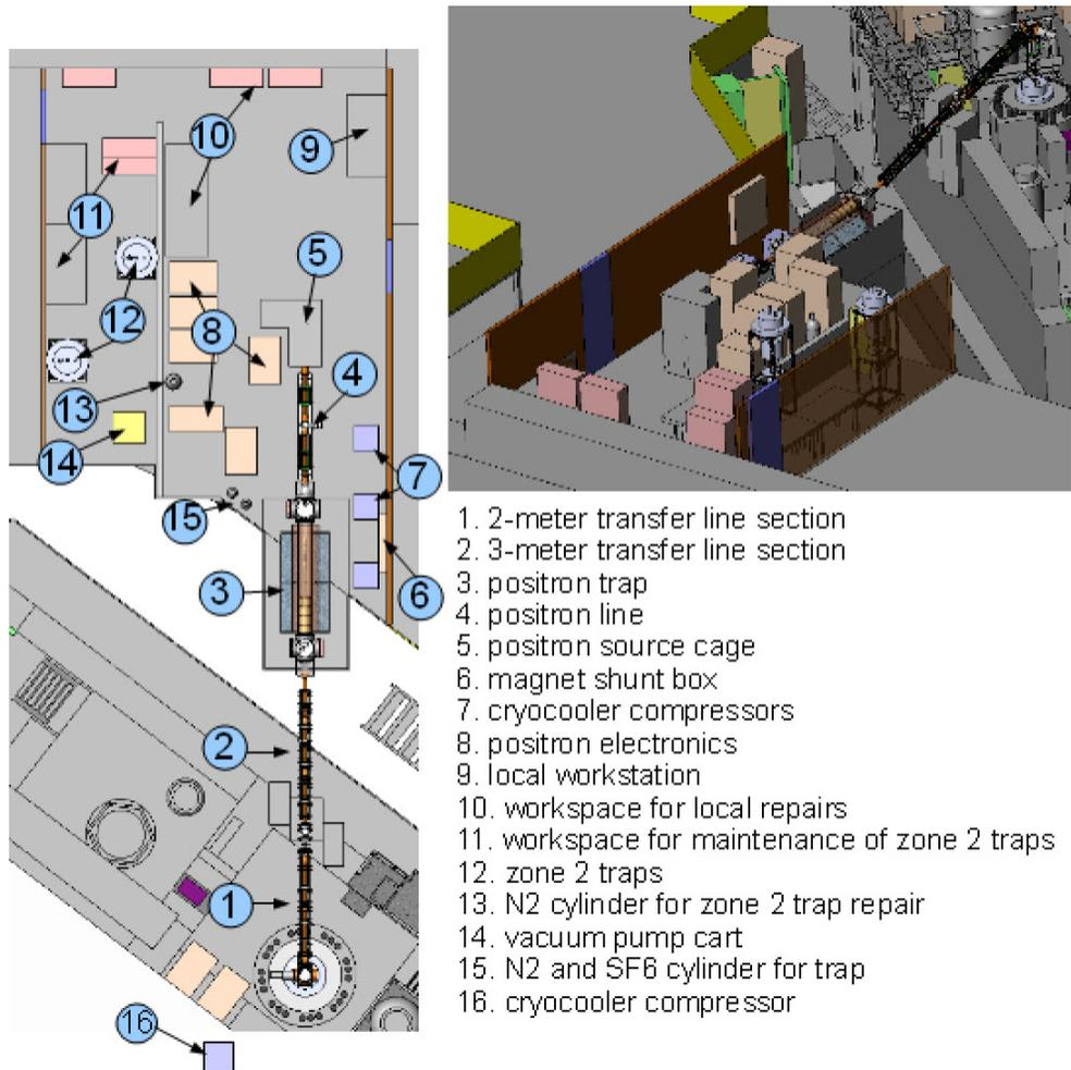
Figure 12: Positron production for antihydrogen production takes place in ATRAP zone 3.
