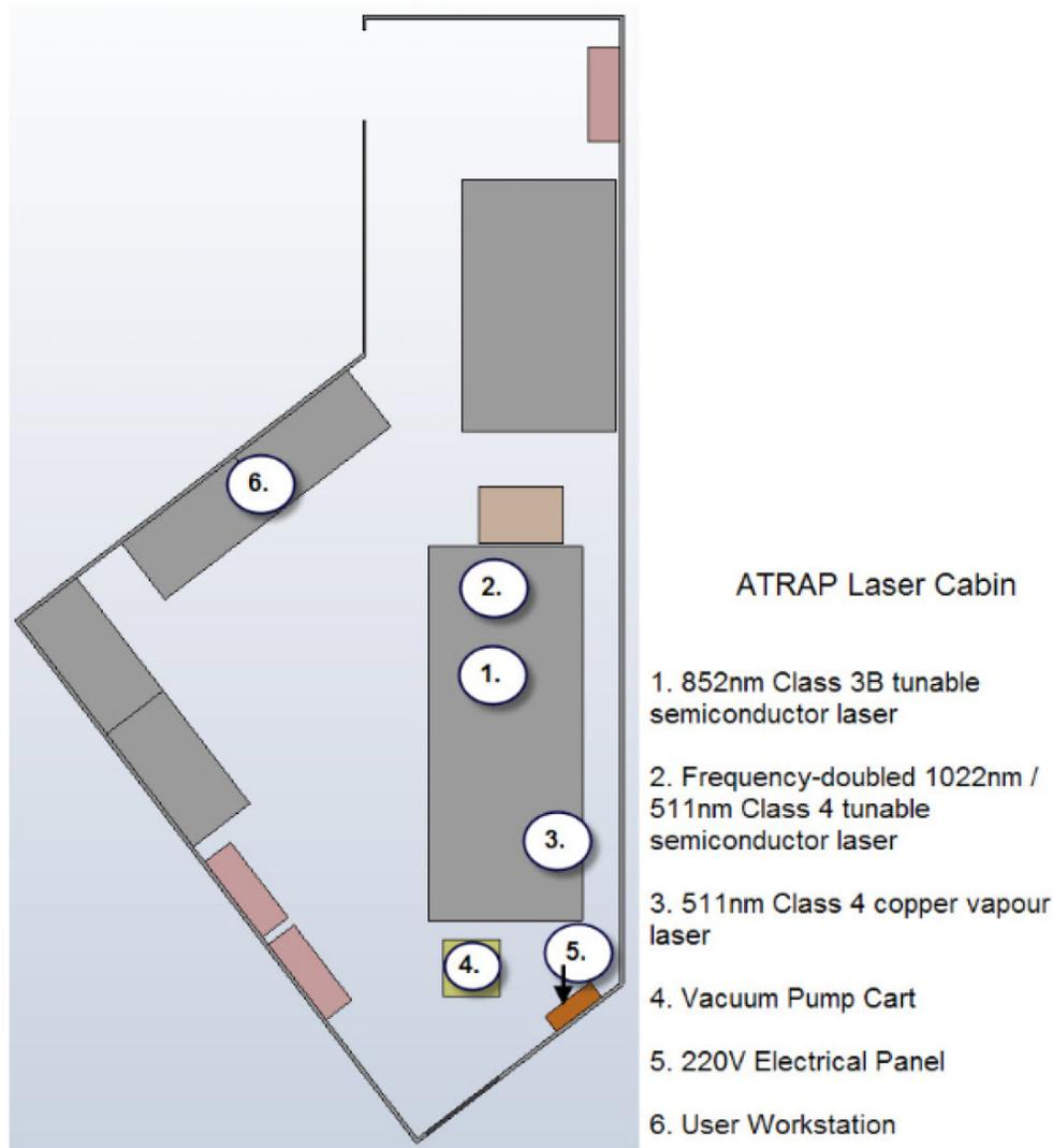
Figure 13: A third Faraday cage contains two laser tables. Our initial laser configuration shown has just been updated to accommodate the pulsed Lyman alpha source described and pictured in the text.
