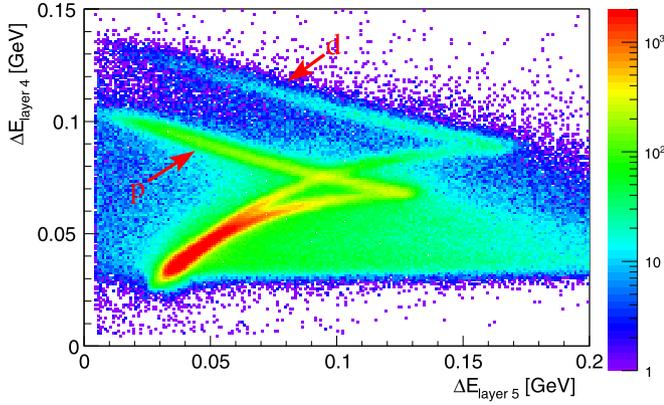
**Fig. 1.** Plot of the energy loss  $\Delta E_{\text{layer } 4}$  of particles in layer 4 of the segmented Range Hodoscope versus that in layer 5 ( $\Delta E_{\text{layer } 5}$ ). The bands of stopped and punch-through protons and deuterons are indicated.
