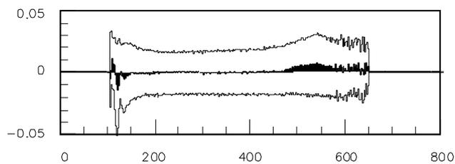
Fig. 1: Example of the drift chamber (DC 1) calibration spectrum.  $\Delta X$  as a function of the drift time.
