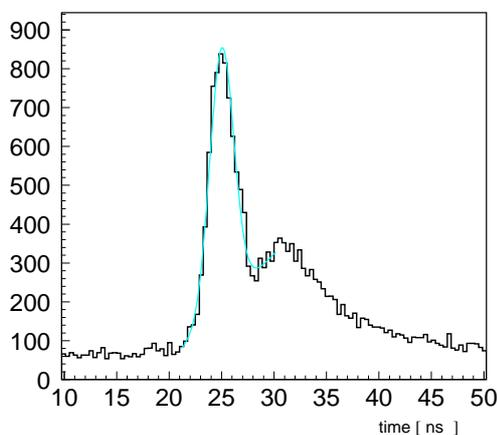
Fig. 2: Time-of-flight determined between the target and the neutron detector.
