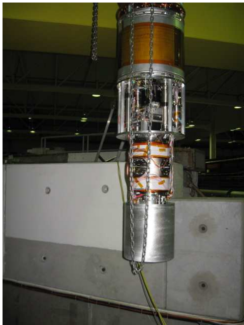
Fig. 1: The BTRAP-experimental set-up showing (from top to bottom) the liquid He dewar, the xy-table, the Ioffe-trap, and the new \bar{p} solenoid.
