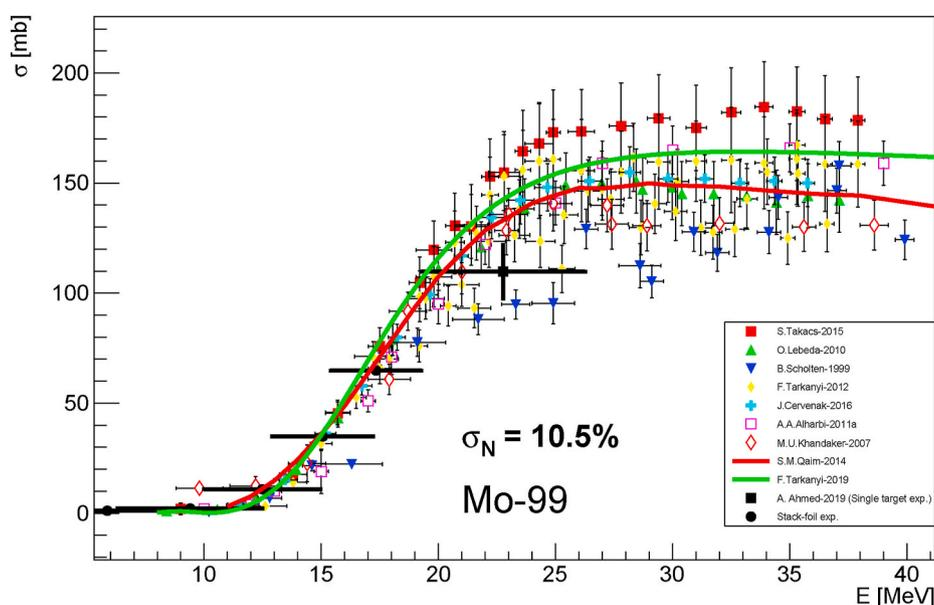
**Fig. 4.** Production cross section of  $^{100}\text{Mo}(p, x)^{99}\text{Mo}$  reactions. The horizontal error bars represent the range of energy degradation within the  $^{nat}\text{Mo}$  target (eq. (4)), and the vertical ones the point specific cross-section uncertainty (see sec. 2.3). The  $\sigma_N$  represents the uncertainty of absolute normalisation.
