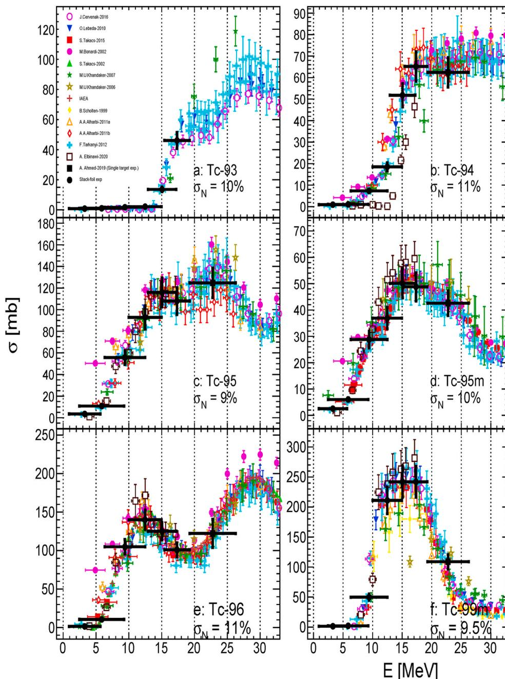
**Fig. 2.** Obtained production cross sections of  $^{nat/100}\text{Mo}(p,x)$  reactions (black circles) shown together with other existing data sets. The horizontal error bars represent the range of energy degradation within the  $^{nat}\text{Mo}$  targets (eq. (4)), and the vertical ones the point specific cross-section uncertainty (see sec. 2.3). The uncertainty of absolute normalisation  $\sigma_N$  is stated in each panel.
