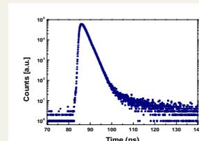
Fig. 4. Fluorescence decay time spectrum in plastic scintillator containing PPO and POPOP compounds.
