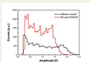
Fig. 3. Cs-137 energetic spectra of plastic and organic crystal scintillator.
