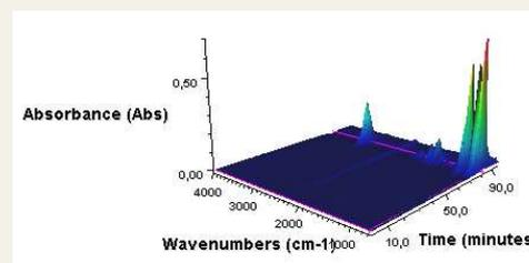
Fig. 8. TG-IR spectrum of a scintillator sample
