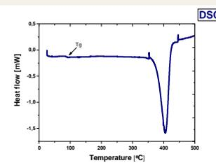
Fig. 7. DSC curve of a scintillator sample.
