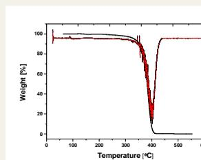
Fig. 6. TG and DTG curves of a scintillator sample.
