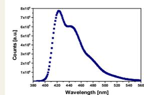
Fig. 5. Emission spectrum of the scintillator with POPOP wavelength shifter.
