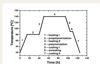
Fig. 2. Temperature cycle steps during plastic scintillators synthesis.
