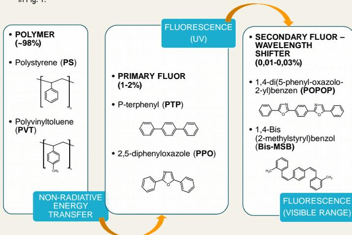
Fig. 1. Energy transfer scheme in a plastic scintillator.
