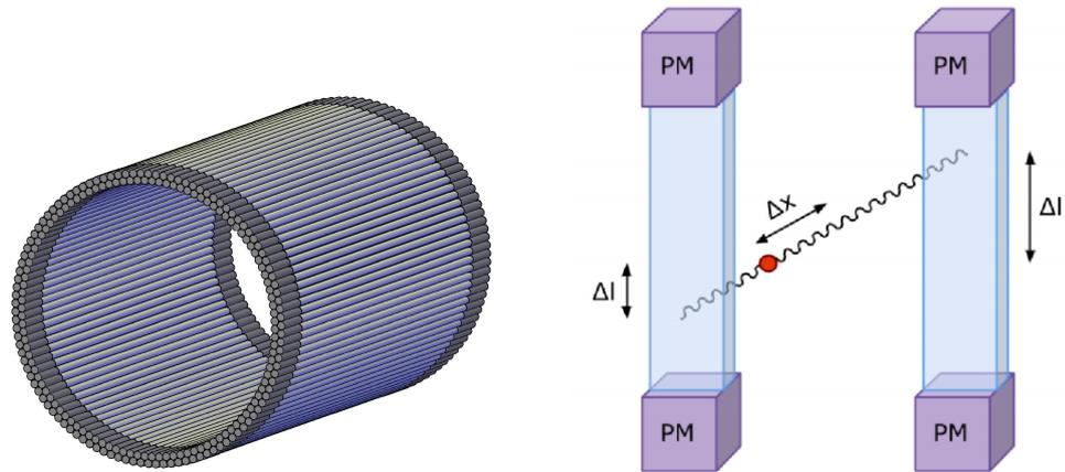
(a) Schematic view of the J-PET diagnostic chamber.
