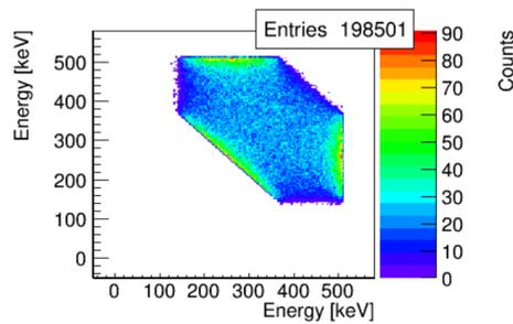
(e)  $E_1$  vs  $E_2$  for events in which each gamma quantum deposited in the detector at least  $50\text{keV}$ .
