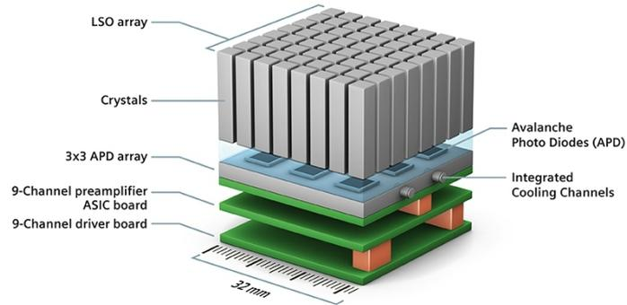
**Figure 2.1:** Block of scintillating crystals (4 x 4 x 20 mm) from Siemens Biograph mMR - PET/MRI scanner. The figure is adapted from Siemens web page.
