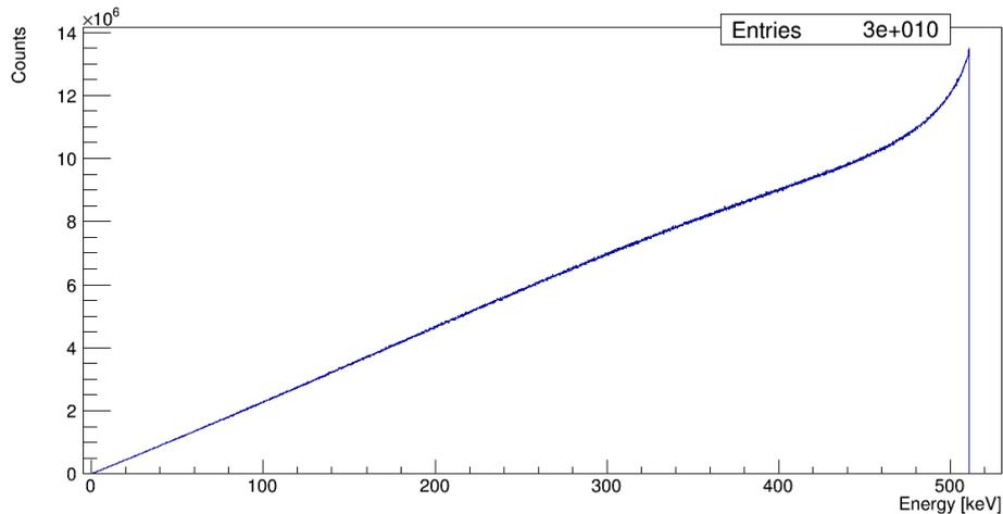
**Figure 5.3:** Energy distribution of single gamma particle originating from the  $\text{o-Ps} \rightarrow 3\gamma$  decay.
