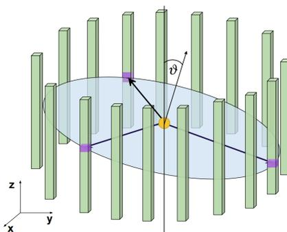
**Figure 6.2:** Decay plane and normal vector.
