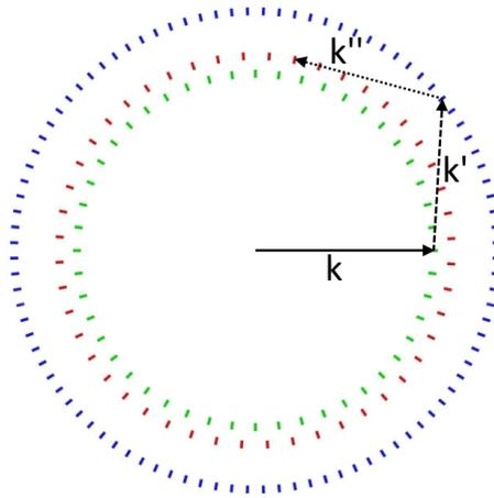
**Figure 6.4:** Schematic illustration of gamma particle scatterings in the detector. Primary gamma particle is gamma scattered once in a detector (vector  $k$ ). Secondary gamma (vector  $k'$ ) is a particle scattered twice in a scintillators. We do not consider tertiary (vector  $k''$ ) and further scatterings.
