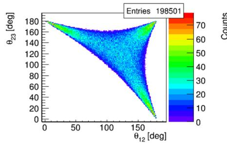
(e)  $\theta_{12}$  vs  $\theta_{23}$  for events in which each gamma quantum deposited in the detector at least  $50\text{keV}$ .
