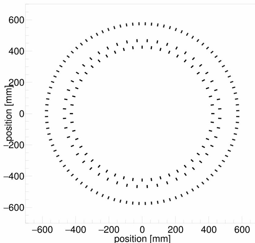
**Figure 5.1:** Projection of all hits onto plane perpendicular to symmetry axis of the J-PET scanner.
