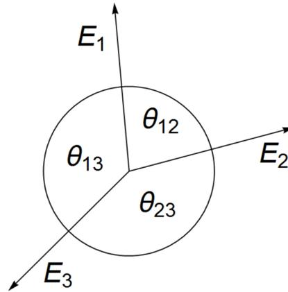
**Figure 5.2:** Schema of  $\text{o-Ps} \rightarrow 3\gamma$  decay.  $E_i$  correspond to energy of  $i$ -th gamma quantum and  $\theta_{ij}$  is an angle between momenta of  $i$ -th and  $j$ -th gamma.
