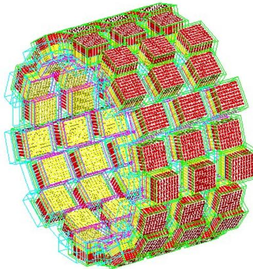
**Figure 2.2:** Schema of scintillator blocks arranged in a detector rings. The figure is adapted from OpenGATE Collaboration web page.
