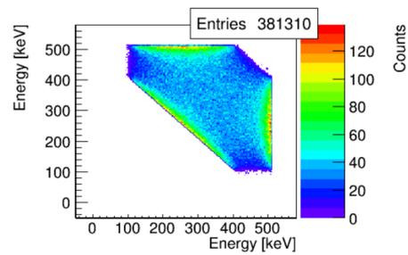
(d)  $E_1$  vs  $E_2$  for events in which each gamma quantum deposited in the detector at least  $30\text{keV}$ .
