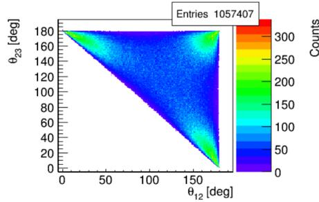
(c)  $\theta_{12}$  vs  $\theta_{23}$  for events in which all three gamma quanta interacted in the detector.
