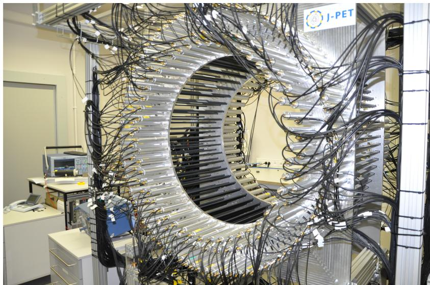
**Figure 2.4:** Photography of mounted prototype. The J-PET detector is made of three cylindrical layers of EJ-230 plastic scintillator strips (black) with dimension of  $7 \times 19 \times 500 \text{ mm}^3$  (192 scintillators in total) and Hamamatsu R9800 vacuum tube photomultipliers (grey). The signals from photomultipliers are probed in the voltage domain at four thresholds with the accuracy of about 30 ps [20]. The figure and caption is adapted from [21].
