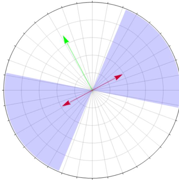
**Figure 3.3:** Plane perpendicular to initial photon momentum. Photon with initial momentum  $511\text{keV}$  is scattered at Compton angle  $\theta = 80^\circ$ . Green arrow is a projection of scattered photon momentum, red arrows represents determined electric field vector and shaded area is area of confidence - area of one standard deviation around determined polarization. In this case that area is equal to  $\pm\sigma = 39.58^\circ$ .
