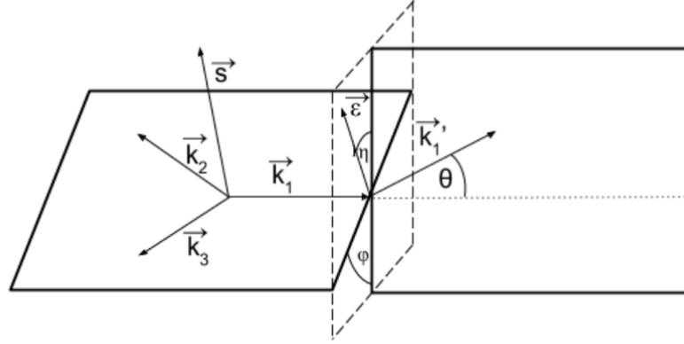
**Figure 3.1:** Schematic illustration of decay plane (the plane spanned on all three photons momentum vectors -  $\vec{k}_i$ ) and scattering plane (formed by momentum vector of primary gamma  $\vec{k}_1$  and scattered gamma  $\vec{k}_1'$ ). Angle  $\phi$  is an angle between those two planes,  $\theta$  is Compton scattering angle and  $\eta$  is angle between scattering plane and linear polarization vector of photon with momentum  $\vec{k}_1$ . Picture adapted from [1].
