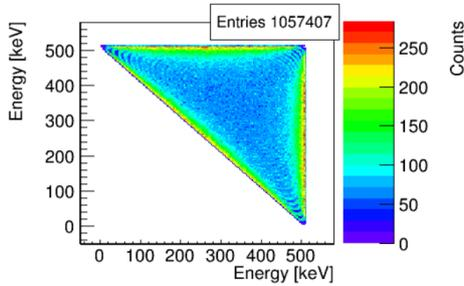
(c)  $E_1$  vs  $E_2$  for events in which all three gamma quanta interacted in the detector.
