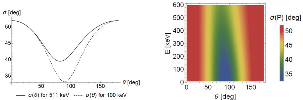
(a) Standard deviation of fig. 3.2 as a function of Compton scattering angle for two chosen energies.
