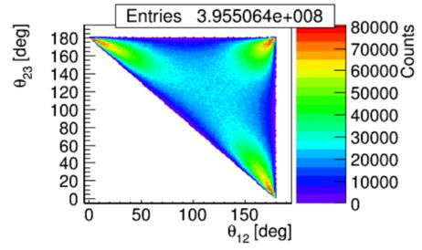
(b)  $\theta_{12}$  vs  $\theta_{23}$  for events in which all three gamma quanta are within geometrical acceptance of the detector.
