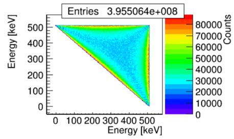
(b)  $E_1$  vs  $E_2$  for events in which all three gamma quanta are within geometrical acceptance of the detector.
