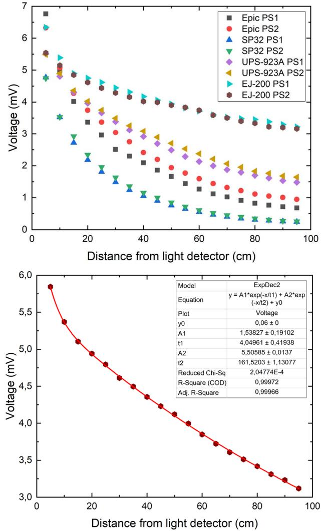
Fig. 2. (Top) Results of the TAL measurements for four types of commercially available plastic scintillators. Two strips of each type were tested. (Bottom) Example of an overlap of the fit  $I(x)$  represented by the red line with the data (black points) for plastic scintillator EJ-200, strip PS1.
