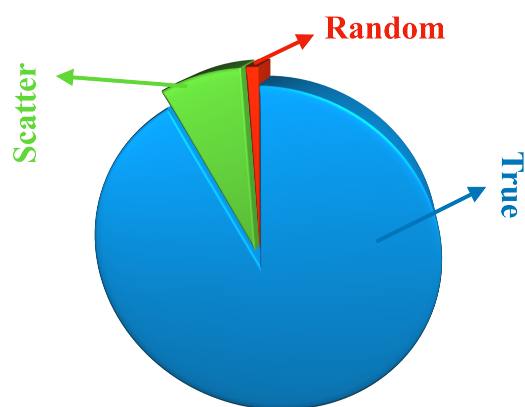
Fig3: Different types of coincidences for sensitivity measurement. The random coincidence rate is 1.1% of true rate.
