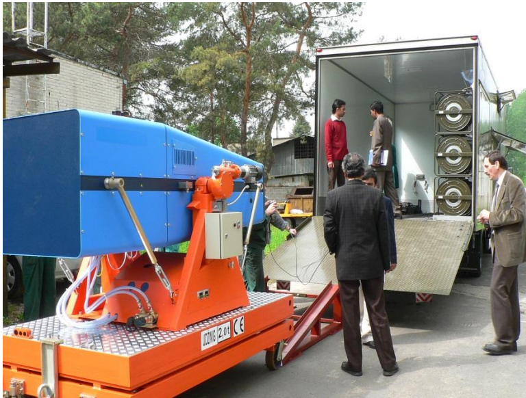
Mobile linac for industrial radiography
