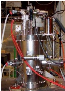
XENON10 Time: Until 2007 xenon: 14kg Fiducial: 5.4kg Limit: \sim 10^{-43}
