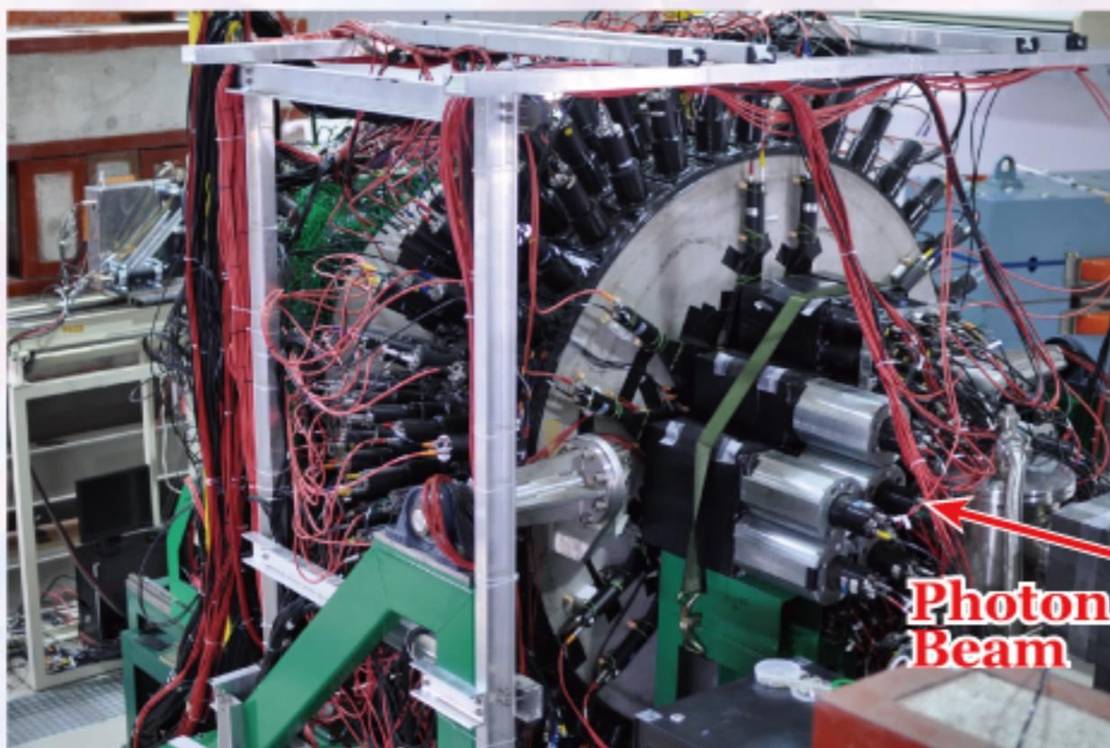
Target: 45 mm thick LH<sub>2</sub> & LD<sub>2</sub>
