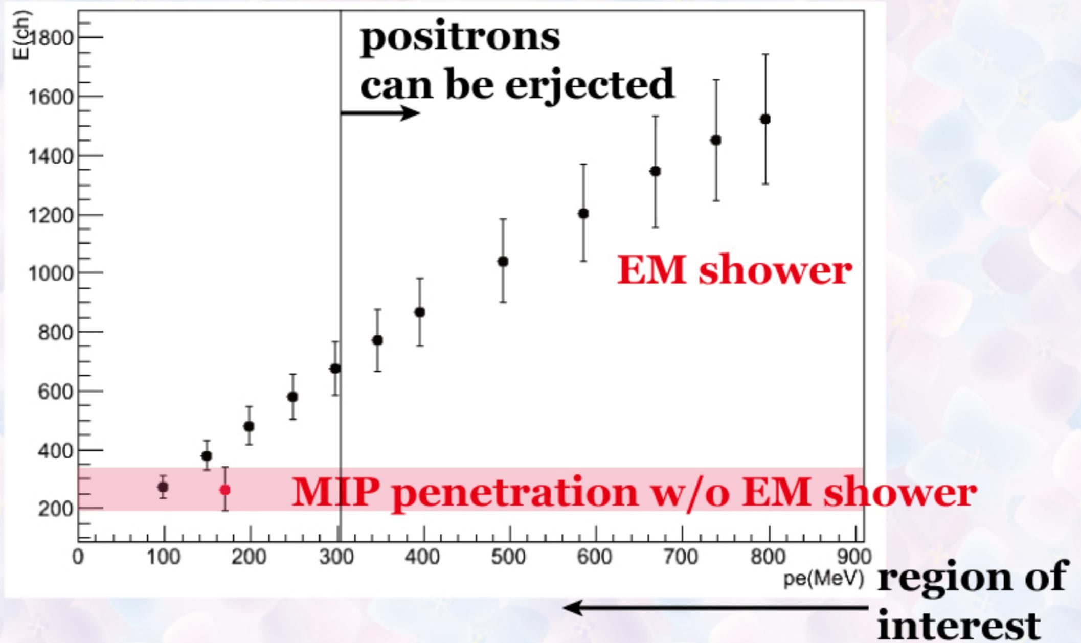
The measured energies in response to the positrons are much higher than those for the charged hadrons.
