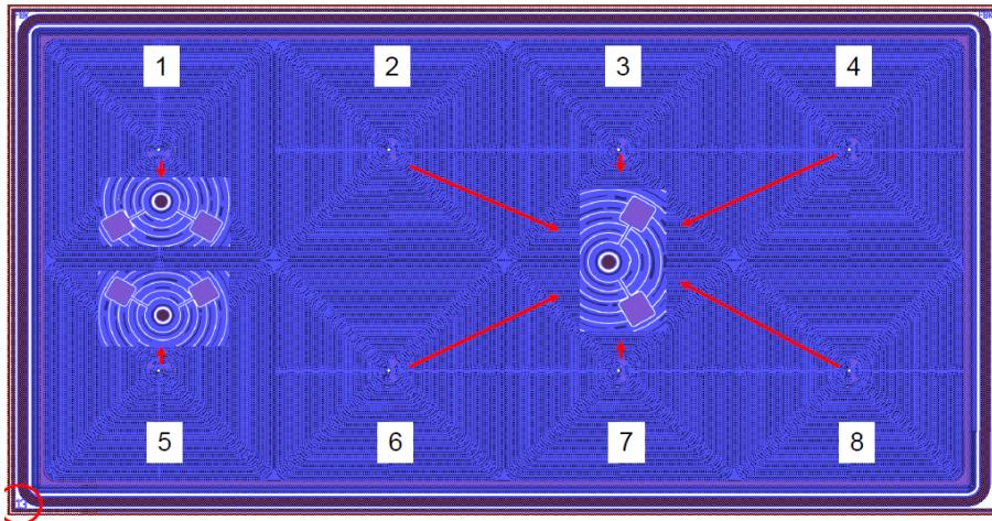
SDD-chip back side with bonding pads
