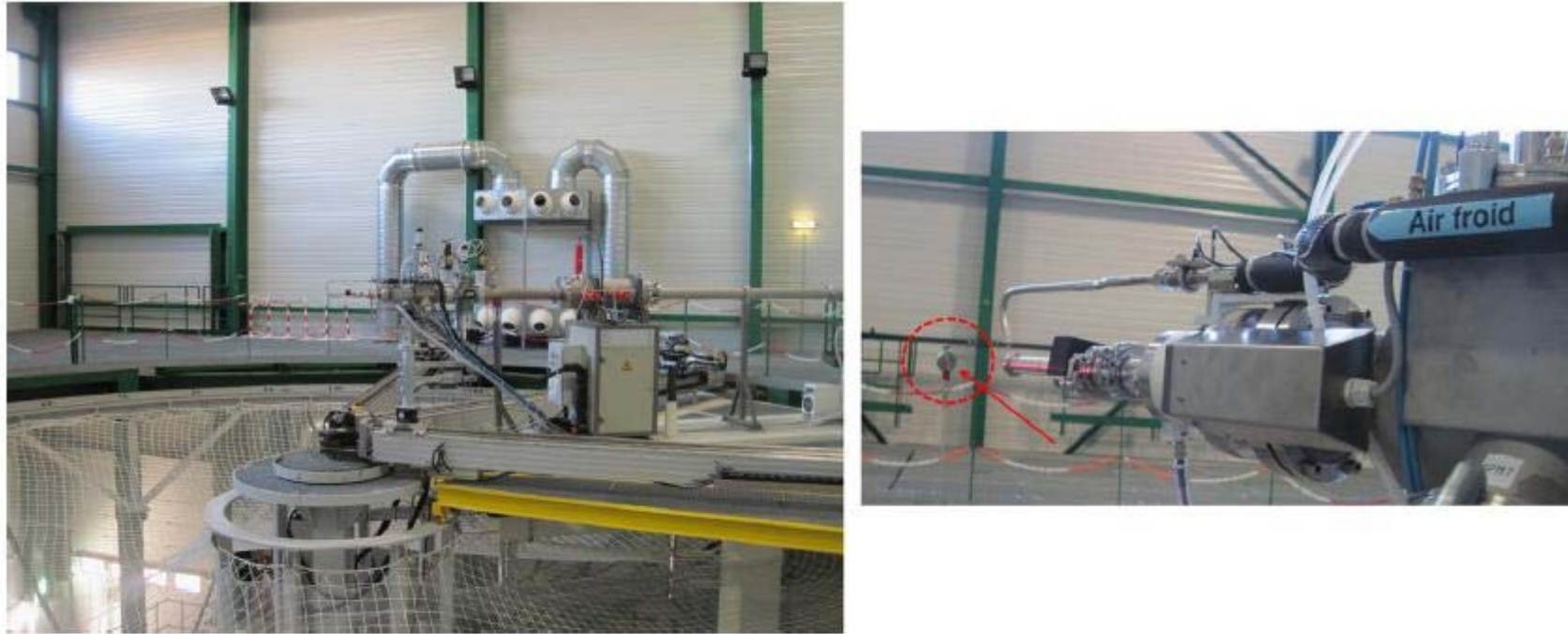
Fig. 1. Photo of the experimental setup showing the end of AMANDE beamline in the low scattering experimental hall (left panel) and the terbium sample (30 mm diameter disk) placed in front of the target (right panel, an arrow directed).
