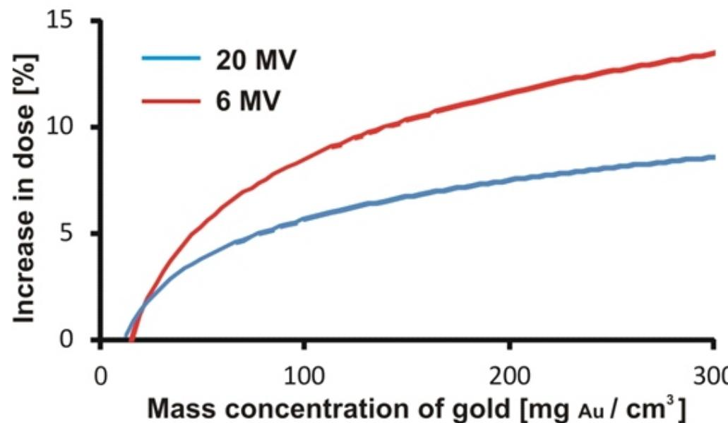
Increase of the dose absorbed in water in the target volume versus the mass concentration of gold in the irradiated medium for the case with the large gold nanoparticles.
