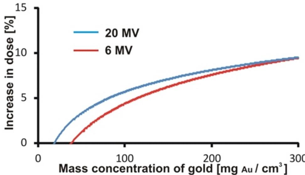
Increase of the dose absorbed in water in the target volume versus the mass concentration of gold in the irradiated medium for the case with the gold atoms.
