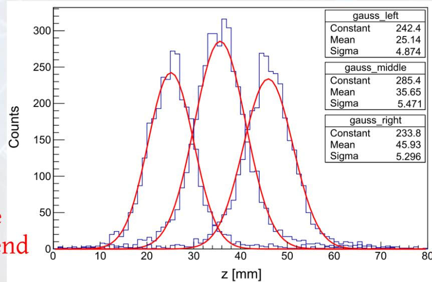
The shape and width of distributions, built from the amplitudes measured in individual WLS strips, depend on depth-of-interaction (DOI) (*yet to measure*)
