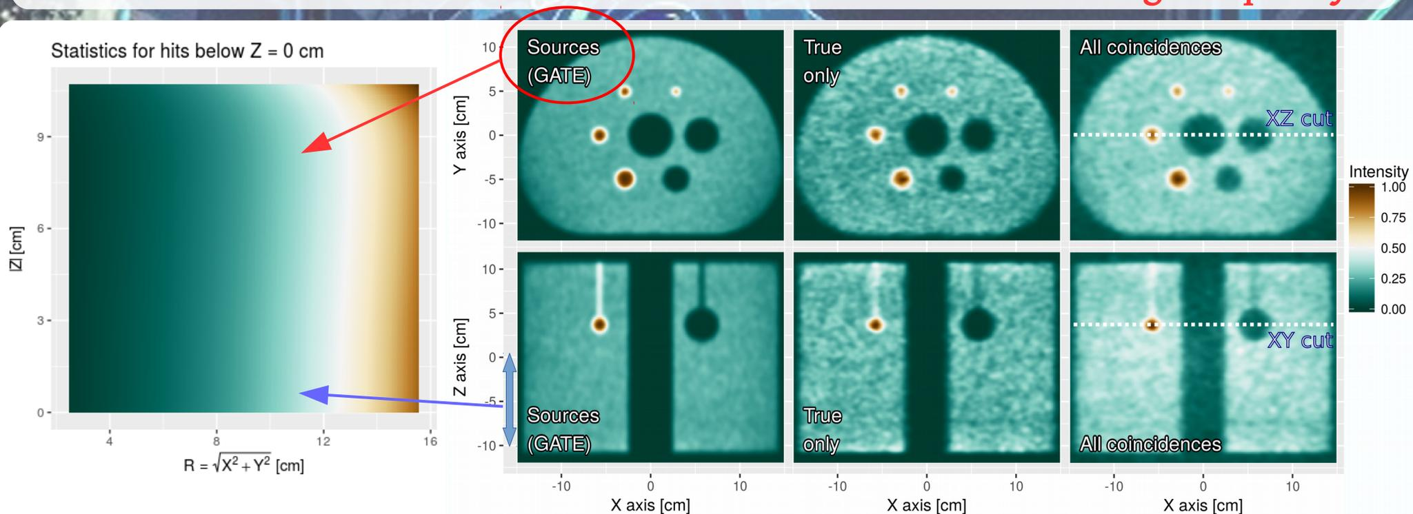
m-KDE/TOF reconstruction (no smearing of  $Z$  and  $t_{hit}$ ). Left: from source positions (in GATE, 6.9 mln. events), centre: from annihilation points for true coincidences (1.9 mln.), right: for all coincidences (4.0 mln.). Elements of bandwidth matrix  $H <$  voxel size (“dscalar”)
