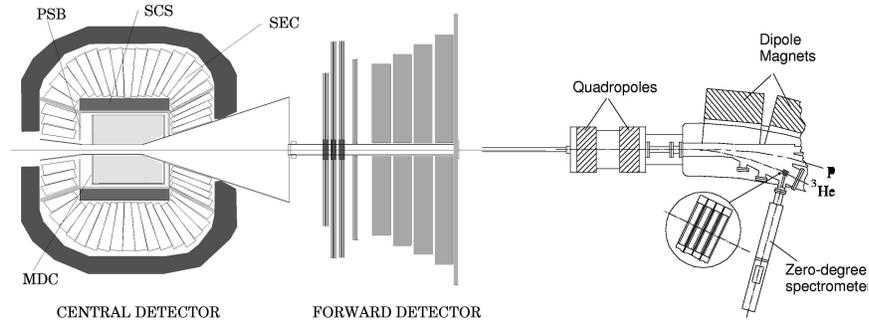
Fig. 2. The cross section of the WASA apparatus with Central Detector built around interaction point, Forward Detector and zero-degree spectrometer. (The scale of the spectrometer's plot was intentionally increased and adjusted to fit the figure.)
