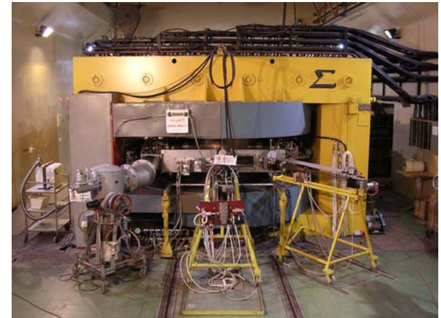
Isochronic cyclotron AIC-144 (1995) 60 MeV protons
