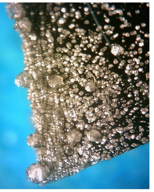
Mono-crystal diamonds about diameter 0.2 mm are grown on Si substrate using the 2%  $C_4 H_{10} / H_2$  composition. The compositions  $C_{6}H_{14}/H_{2}$ is also tested. Diamond detectors are obtained using 7% CH<sub>4</sub>/H<sub>2</sub> compositions.
