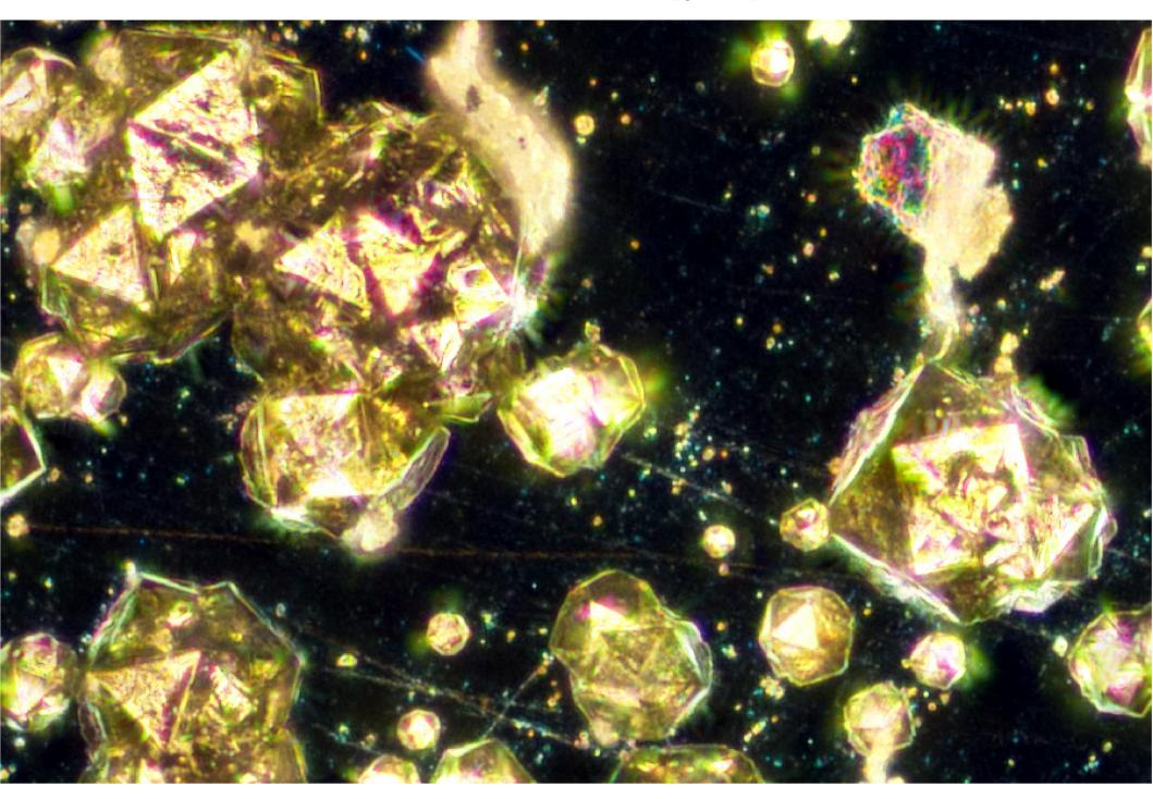
Diamond mono-crystals square pyramides grown on HPHT [100] diamond Sumimoto substrate,  $2\% C_4 H_{10} / H_2$  composition.
