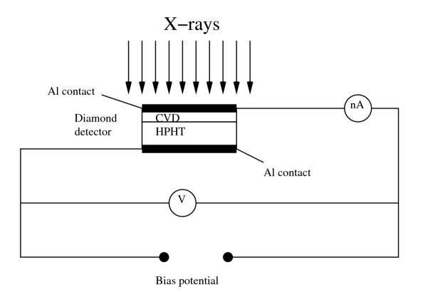
X-ray tube: 40 kV, 10 mA, dose strength at 1 mm<sup>2</sup> diamond detector = 2 Gy/s.
