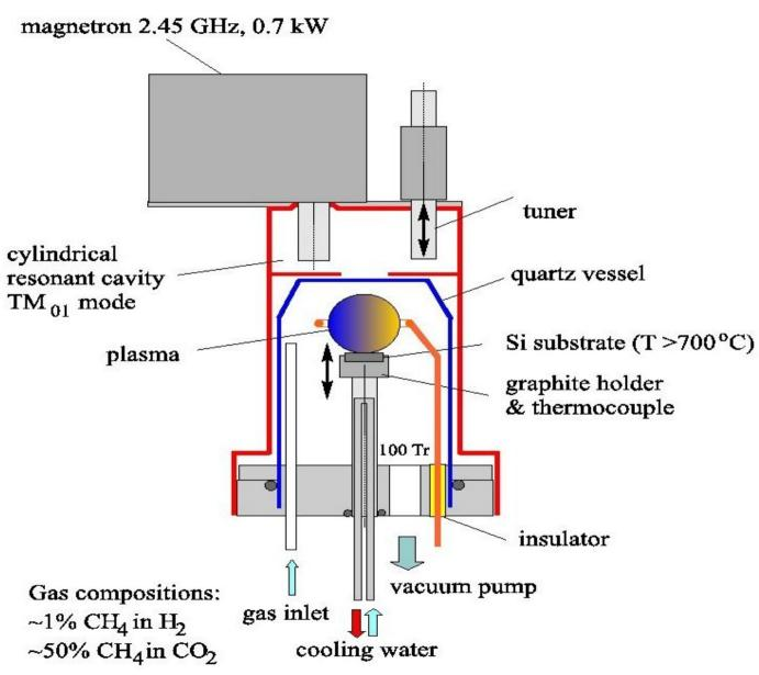
Stabilization systems: - Gases ratio & pressure. - Stabilization of target temp. by: - optical observation of target & - magnetron power regulation. The gases are ionized into active radicals to create diamond and graphite
