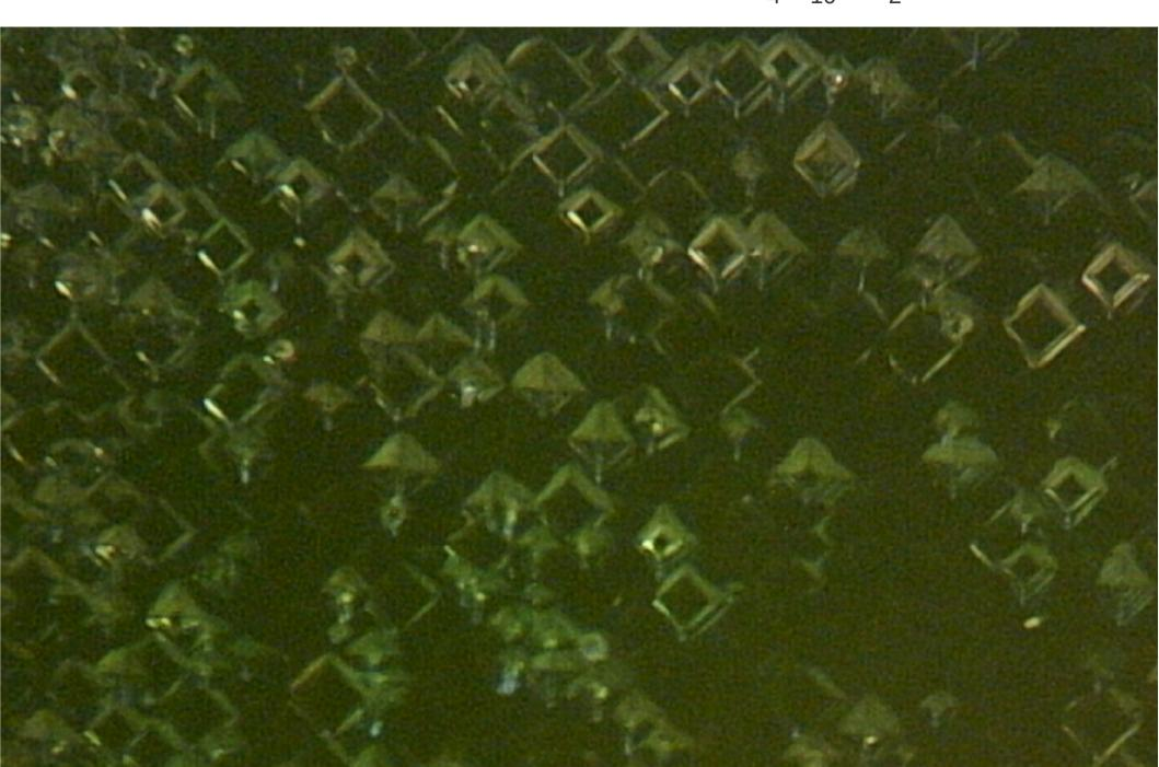
$\mu$ m diamond monocrystal layer grown on HPHT [100] diamond Sumimoto substrate, 7% C<sub>4</sub>H<sub>10</sub> /H<sub>2</sub> composition.
