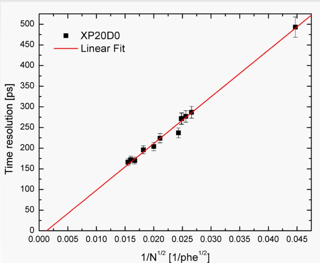
Measured time resolution versus number of photoelectrons ( $N_{phe}$ ) collected in the PMT
