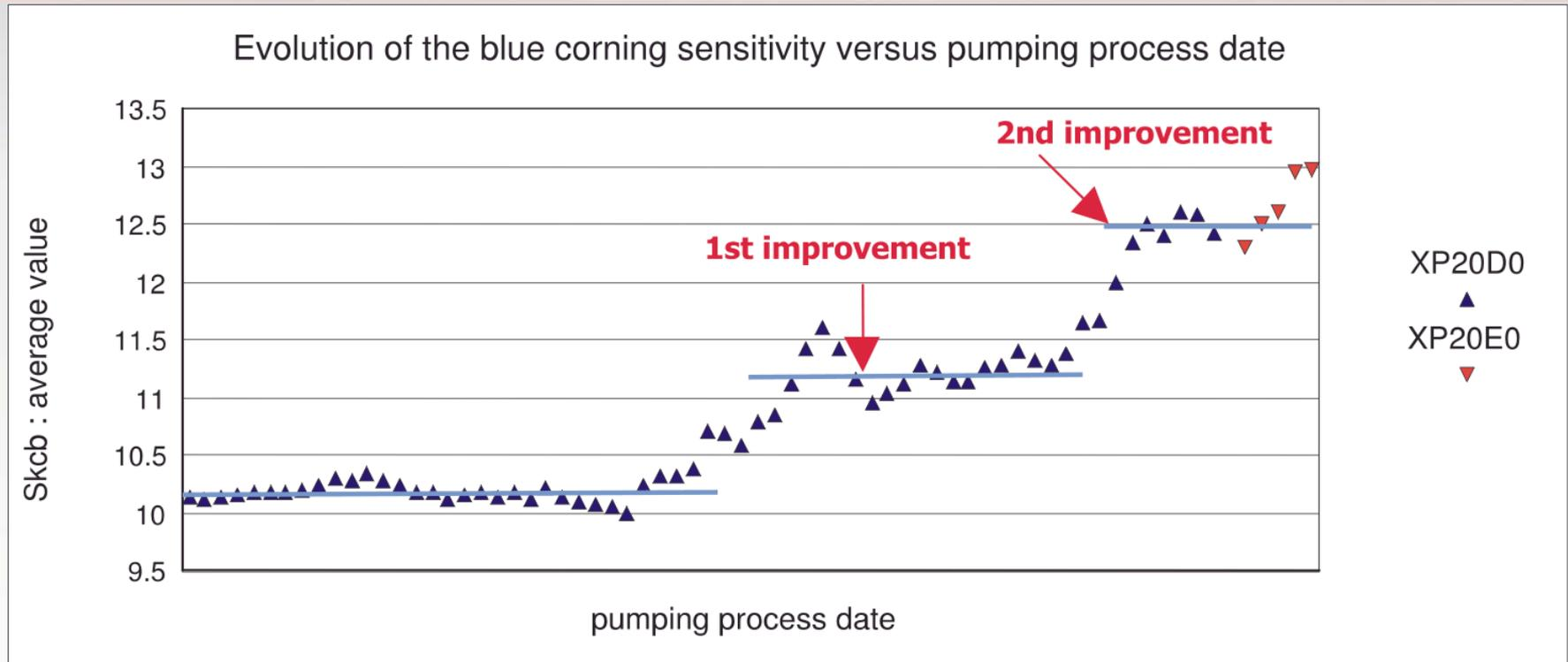
An improvement of the photocathode QE in the XP2020 family. We have tested XP20D0 and XP20E0 with the blue sensitivity close to 14  $\mu\text{A}/\text{lmF}$  (QE up to 35%). The best values - above 40%.
