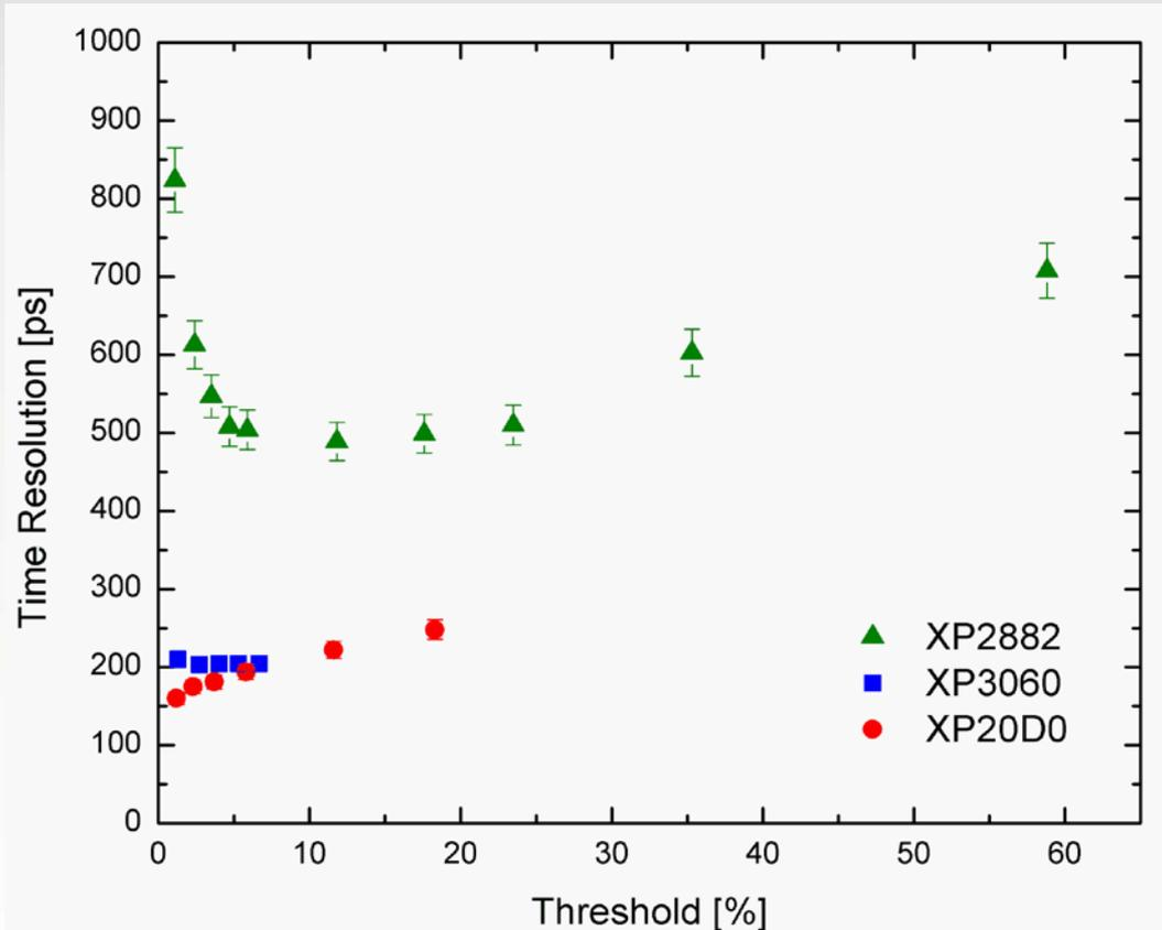
Time Resolution dependence on the LE threshold for PMTs representing different constructions
