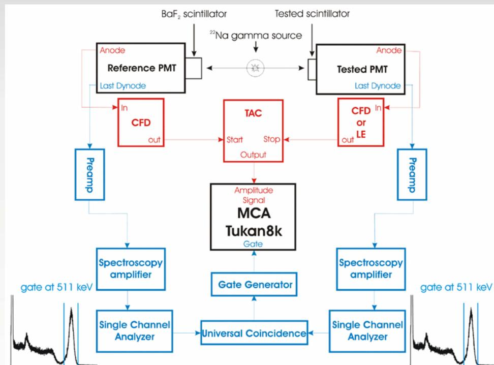
Fig. 2. Experimental setup for timing resolution measurements.
