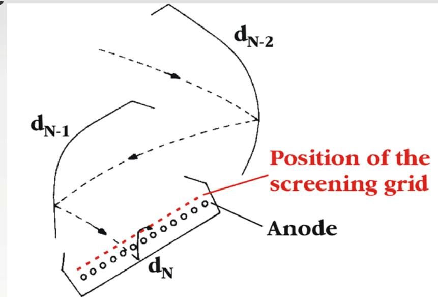
Fig. 2. Geometry of the last dynodes and the anode in a typical linear-focused photomultiplier. Note that the anode is built as a grid inside the last dynode. The position of the screening grid is also shown.
