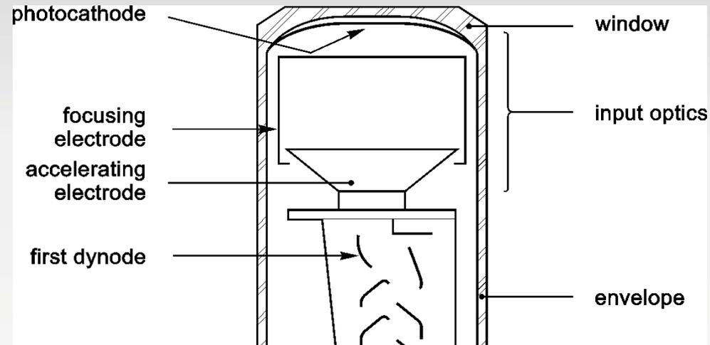
Figure 23 : Cross Section of Metal Channel Dynode with Electron Trajectories
