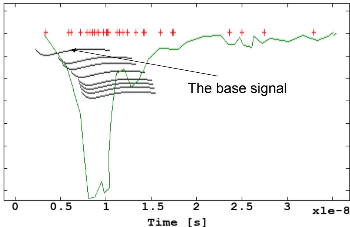
Example base signal for supply voltage of F2 pmt equal 2400V:
