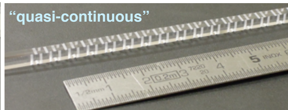
5 mm pitch, four faces staggered
