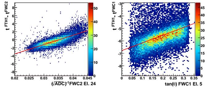
Fig. 2: (a) Experimental data of time-of-flight between FTH1 and FWC2 as a function of  $\sqrt{ADC}^{-1}$  for element 24th of FWC2 with superimposed line  $\Delta t = \alpha \cdot \frac{1}{\sqrt{ADC}} + \beta$  to establish a time "Walk effect". (b) Experimental data of time-of-flight between FTH1 and FWC1 as a function of  $\tan\theta$  for element 4th of the FWC1 with superimposed line  $\Delta t = \alpha \cdot \tan\theta + \beta$  to establish light propagation effects.
