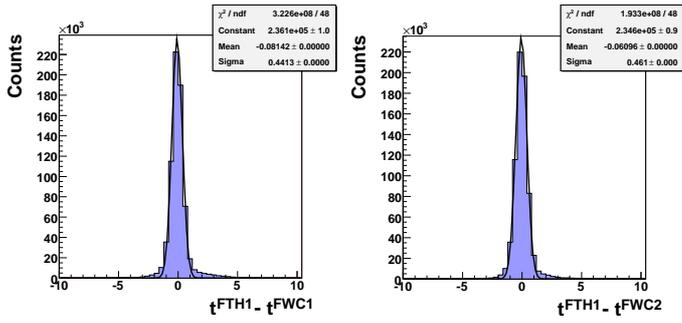
Fig. 3: Experimental data of time-of-flight between (a) FTH1 and FWC1, (b) FTH1 and FWC2 for all modules. The result of the fitted Gauss function is shown as a solid line. Fit parameter  $\sigma$  shows the time of flight resolution.
