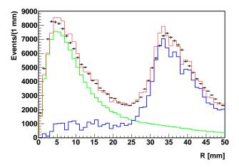
Figure 4: Distribution of the distance R between the COSY beam axis and the reconstructed point of closest approach of  $e^+$  and  $e^-$  tracks: experimental data (black crosses); simulations for  $\pi^0 \to \gamma \gamma$  (blue line), the  $\pi^0 \to e^+e^-\gamma$  decay (green line), and the sum of the two contributions (red line).
