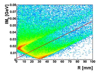
Figure 5: Correlation between R and  $IM_b$  variables for the experimental data. The selection cut is shown by the diagonal line. The events below the line mainly come from photon conversions in the beam pipe.
