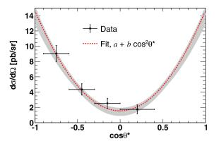
**Fig. 2.** Angular distribution of the  $dd \to {}^4{\rm He}\pi^0$  reaction at Q=60 MeV. The result of the fit up to second order in  $\cos\theta^*$  is shown with a dotted curve. The systematic errors of the fit are presented as a gray band. The horizontal error bars indicate the bin width.
