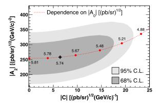
**Fig. 4.** Correlation plot for the parameters |C| and  $|A_2|$  determined from the fit of the angular distribution of  $dd o {}^4{\rm He}\pi^0$  at Q=60 MeV. The center point marked with the cross shows the result from Eq. (6). The shaded areas indicate the 68% and 95% confidence regions. The dotted line shows the influence of a variation of  $|A_0|$  on |C| and  $|A_2|$ , with the circle points representing the results for the indicated values of  $|A_0|$ .
