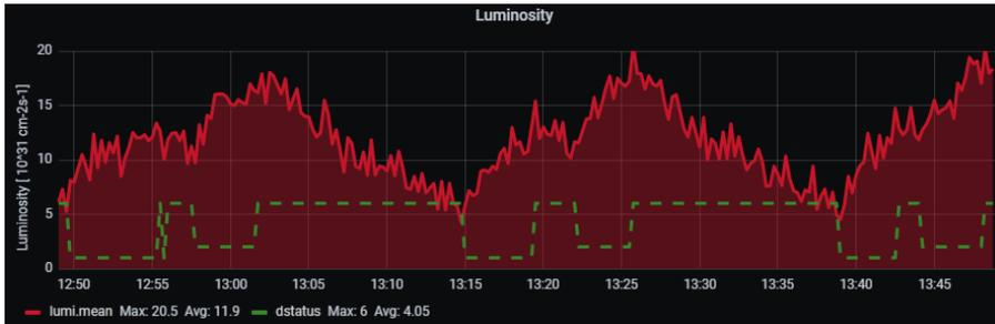
Figure 7: The estimated instantaneous luminosity, in units of  $10^{31} \text{ cm}^{-2}\text{s}^{-1}$ , for one hour of the kaonic helium data on 6 May 2023. The status of the accelerator in the same period - dashed green line.
