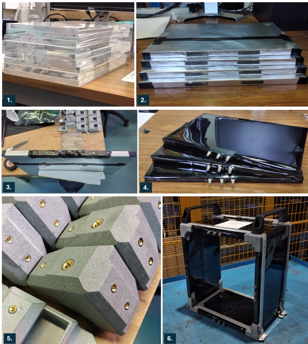
Figure 12. Construction process of the SARA scintillation detector. 1. Some of the polished scintillator panels. 2. Some scintillators wrapped in aluminum. 3. A PCB applied on a scintillator. 4. Three scintillators wrapped in OPAQ-1152i. 5. Some corner elements with ensats. 6. The first completed box.
