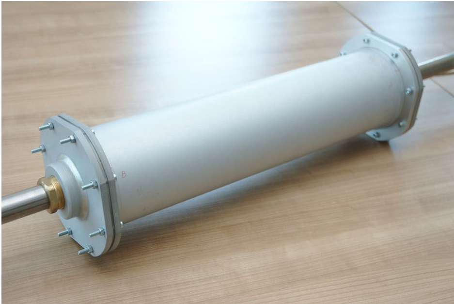
Run 3 chamber, R \approx 7 cm No o\text{-Ps} production medium 2 days of measurement
