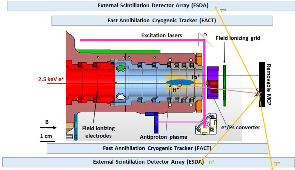
**Figure 3:** Updated scheme for antihydrogen production in AEGIS Phase 2.
