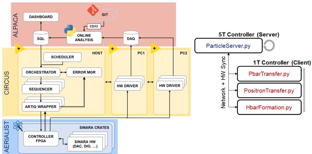
Figure 2: Architecture of the AEGIS control system
