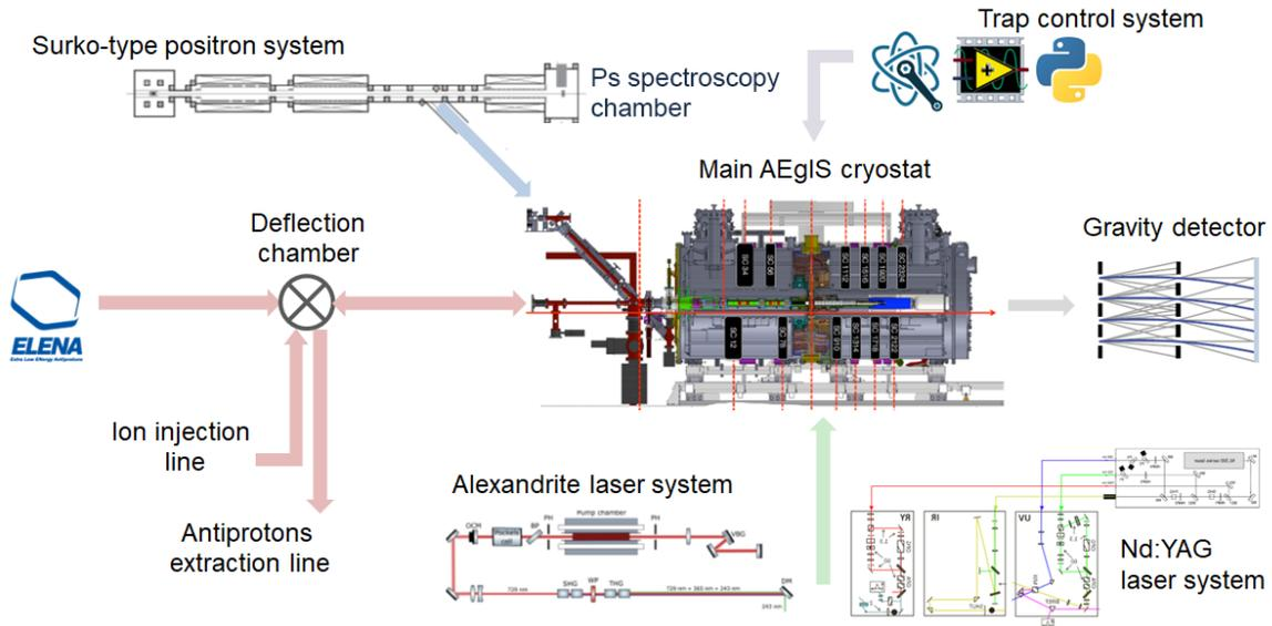
**Figure 1:** Overview of the AEGIS experimental setup as of 2024. The key components include the main cryostat, positron system, laser system, and detection arrays, as well as the control system for coordinating operations.
