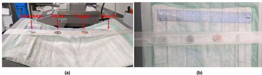
**Fig. 9** Photographs of an experiment used to measure the quartz-glass o-Ps lifetime using  $^{68}\text{Ga}$ . Drops of the  $^{68}\text{Ga}$  solution were placed on each disk shown in (a). Another disk of the same material was then placed on top and the two disks were taped together as shown in (b)
